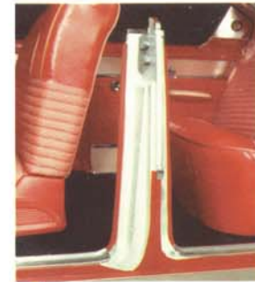
Mercury Phaeton's sturdy side pillars are reinforced by an additional bracing running from pillar to pillar.
