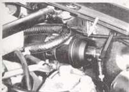
Ignition coil left: Terminal 1 and 15, High tension ignition lead term. 4
