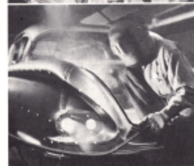
Body joints are spot welded.
