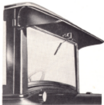
One-piece windshield with automatic wiper.
