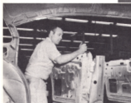
Door window is fitted into place.
