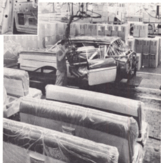
Seats are placed in position as the bodies glide down the line.
