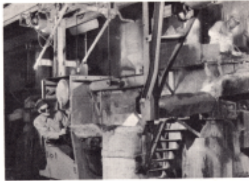
Pouring of hot metal from cupola into ladle at foundry.
