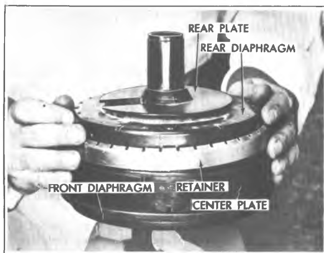
Fig. 5-11B—Installing Rear Diaphragm Retainer
