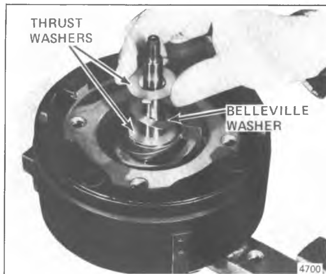
Figure 1D-105 Replacing R-4 Thrust and Belleville Washers
