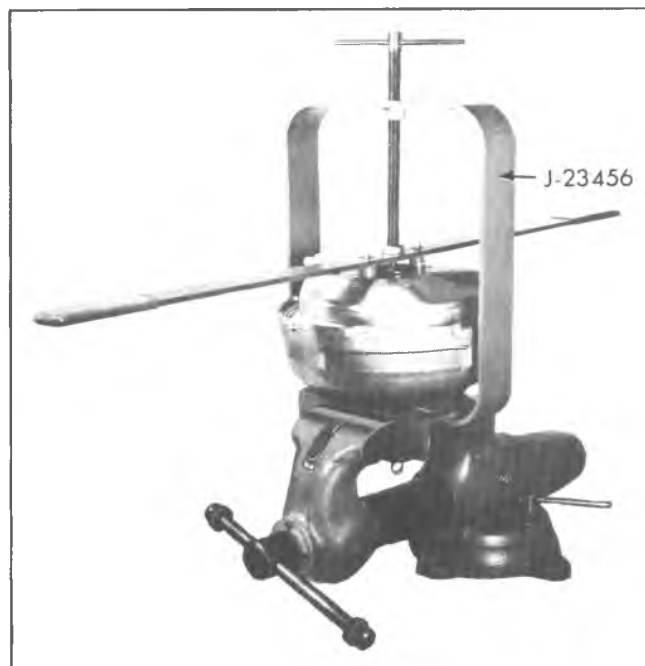
Fig. 5-1A—Unlocking Front and Rear Housings
