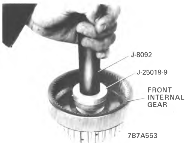
Figure 7A1-192 Installing Front Internal Gear Bushing
