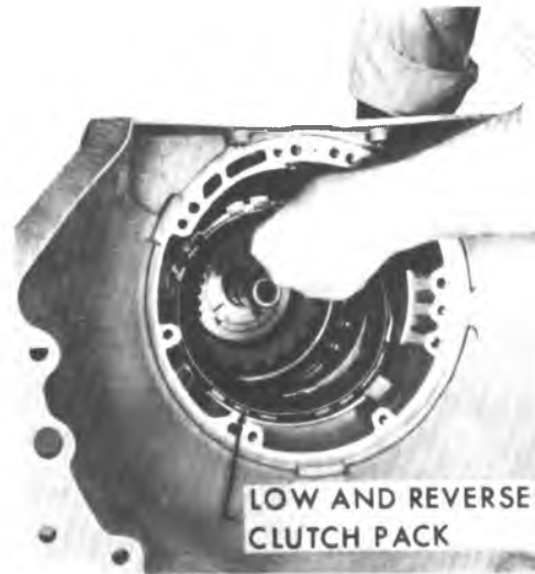
Figure 7A5-34 Low & Reverse Clutch Plate Removal
