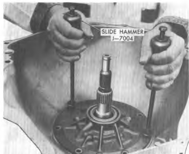
Figure 7A5-23 Pump Removal
