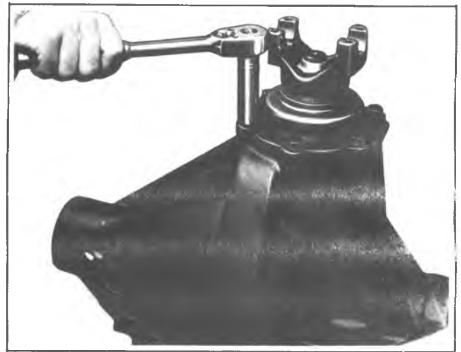
Fig. 7E—Removing Retainer Bolts
