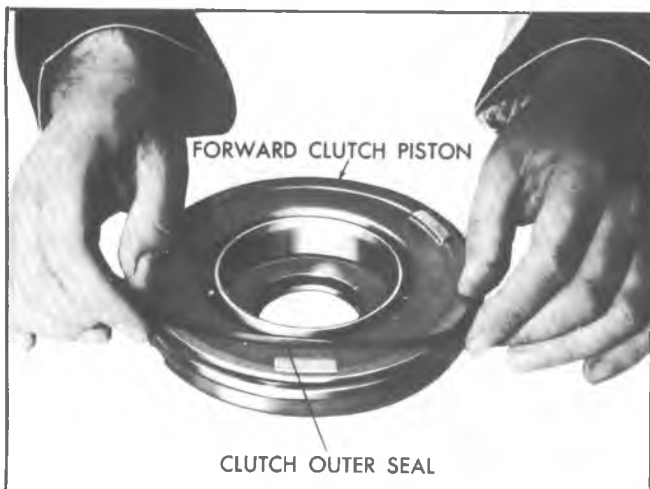
Fig. 7A-84C--Removing Forward Clutch Piston Outer Seal
