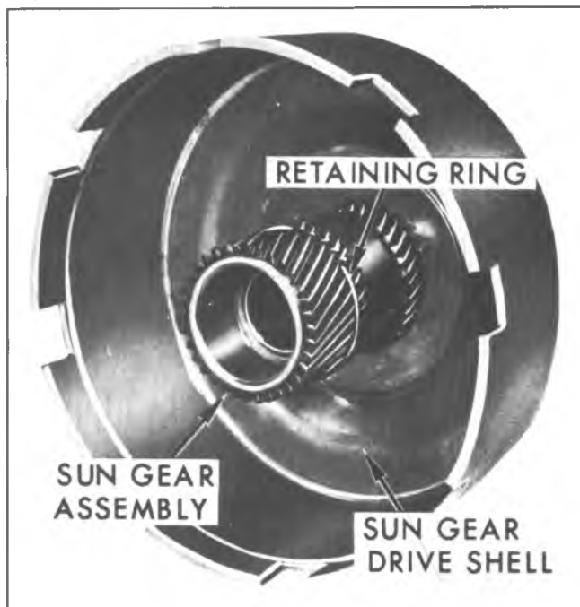
Fig. 7A-92B--Removing Sun Gear to Drive Shell Front Steel Thrust Washer
