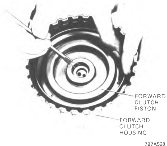
Figure 7A1-130 Installing Forward Clutch Piston
