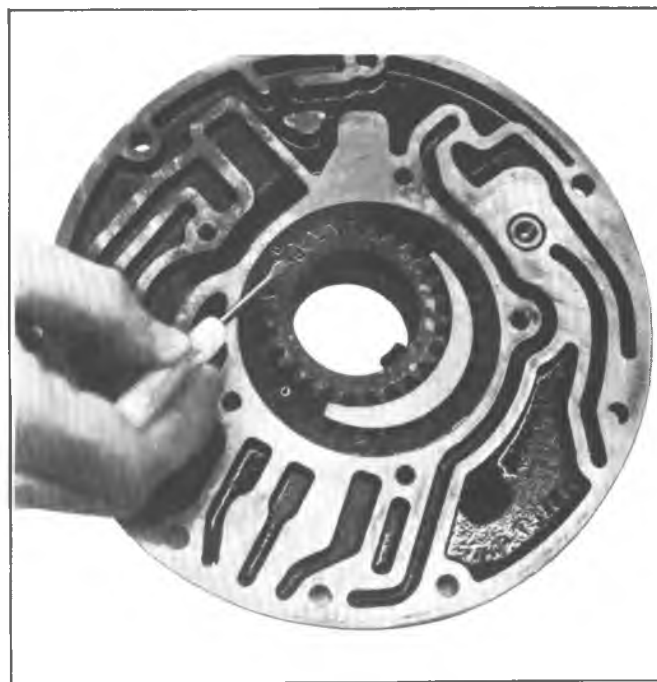
Fig. 7A-66B--Installing Pump Drive and Driven Gears
