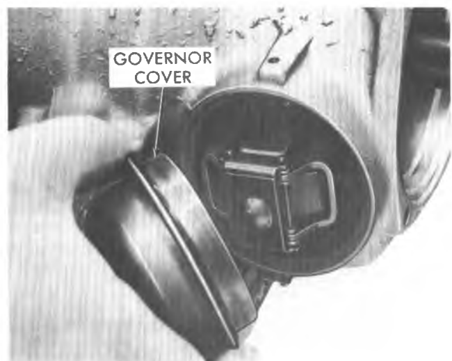
Figure 7A5-15 Governor Cover and "O" Ring Seal
