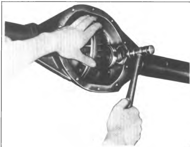
Fig. 9B--Installing Differential Shim
