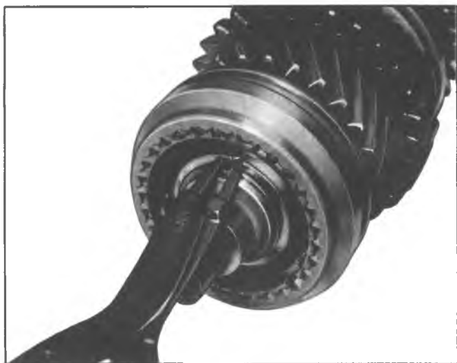
Fig. 7B-7A—Removing 2nd-3rd Clutch Hub Retaining Ring
