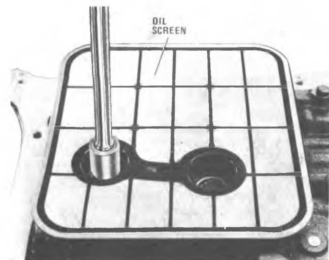
Figure 7A1-17 Removing Oil Screen
