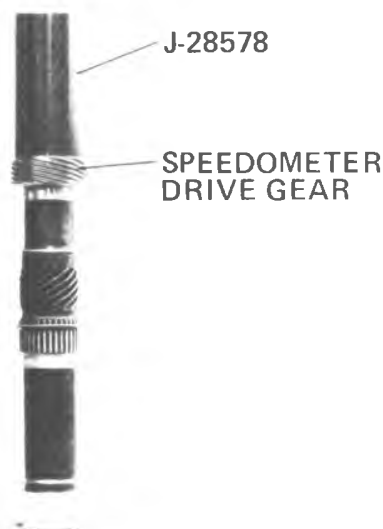
Figure 7A1-74 Installing Speedo Gear (Steel)
