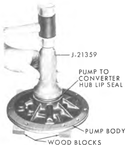
Figure 7A5-48 Installing Hub Lip Seal
