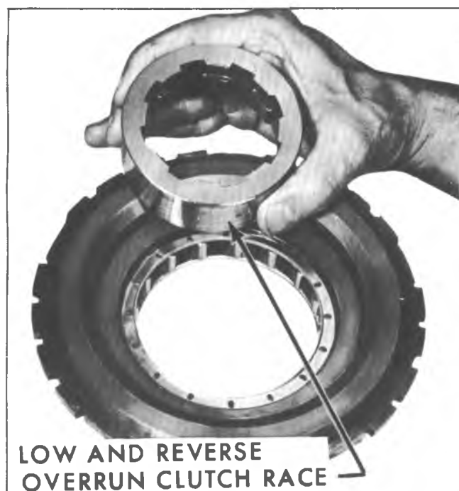
Fig. 7A-94B--Removing Overrun Clutch Inner Race
