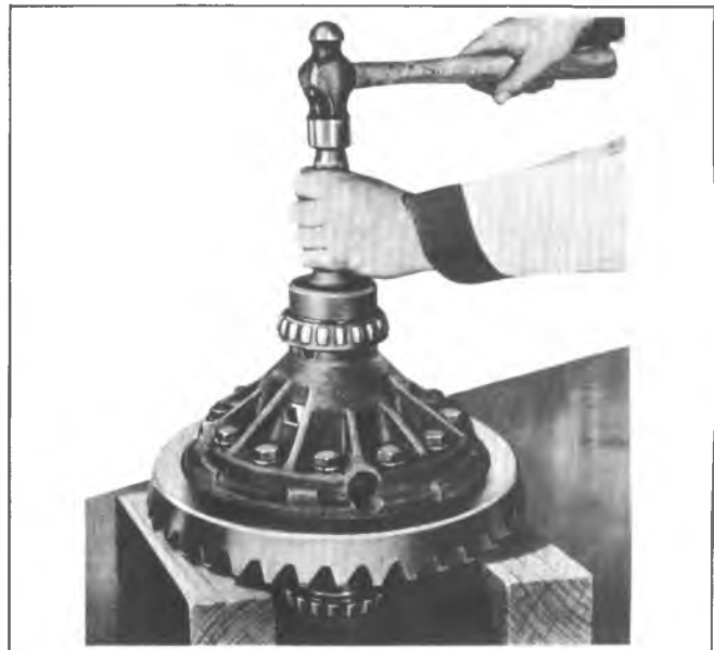
Fig. 5E-Differential Bearing Installation
