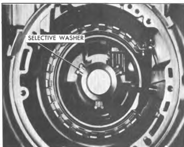
Fig. 7A-43C--Removing Selective Washer
