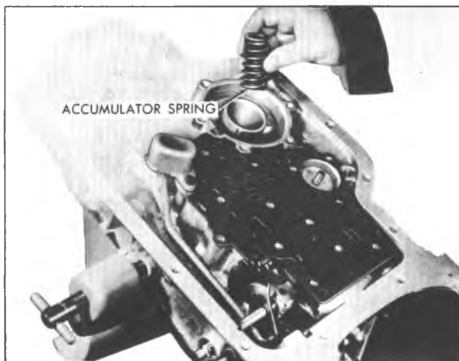
Fig. 7A-180C--Installing Rear Accumulator Spring
