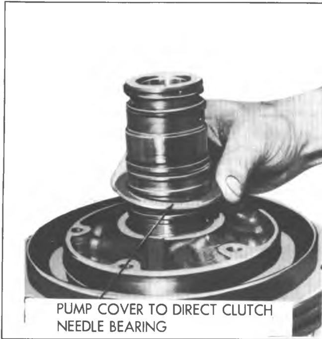
Fig. 7A-108B--Pump Cover to Direct Clutch Torrington Bearing
