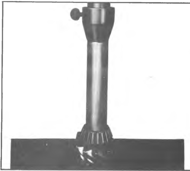
Fig. 22B—Installing Rear Bearing
