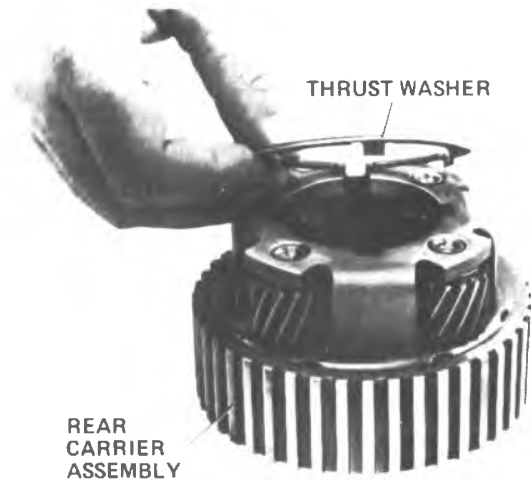
Figure 7A1-83 Installing Thrust Washer
