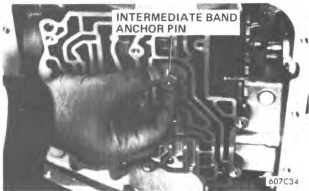
Figure 7A1-156 Installing Intermediate Band Anchor Pin
