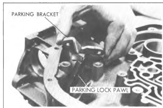
Fig. 7A-23C--Removing Parking Bracket
