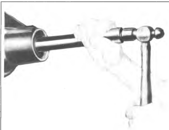
Fig. 17B—Installing Pinion Front Bearing Cup
