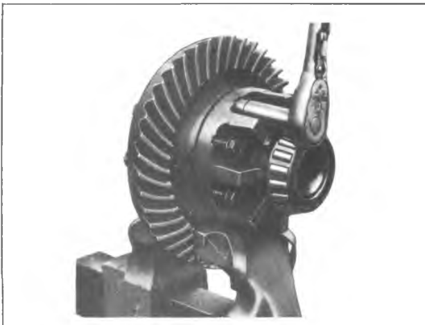
Fig. 3F—Separating Case Halves
