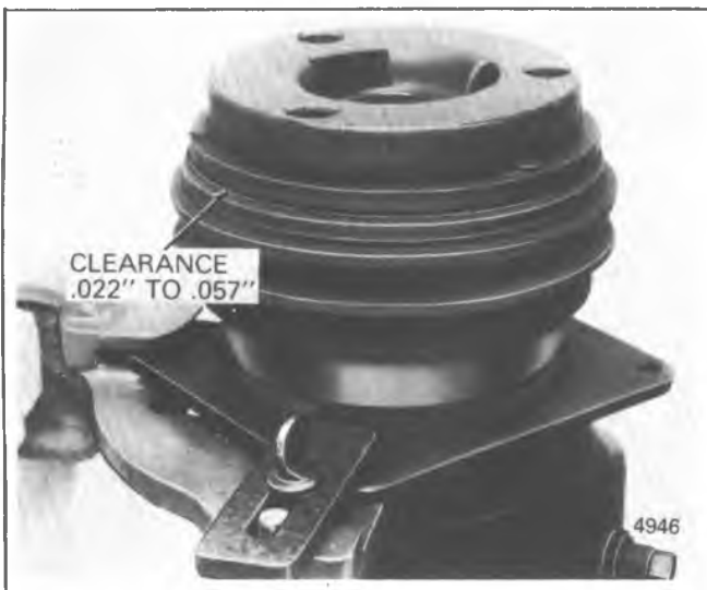
Figure 1D-11 Checking A-6 Air Gap
