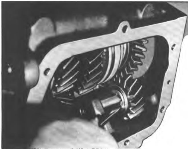
Fig. 7B-3A--Removing Reverse Idler Shaft "E" Ring
