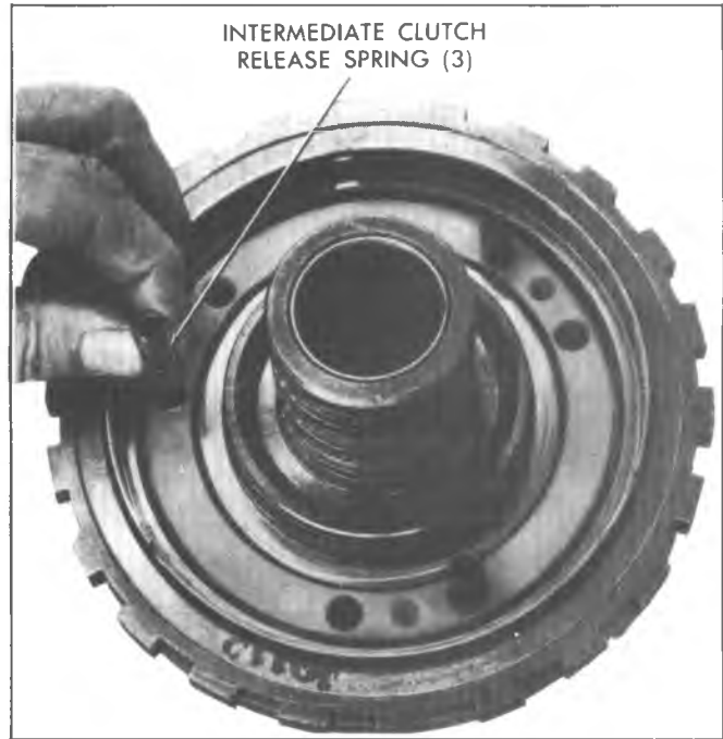
Fig. 7A-115C--Removing Clutch Release Springs
