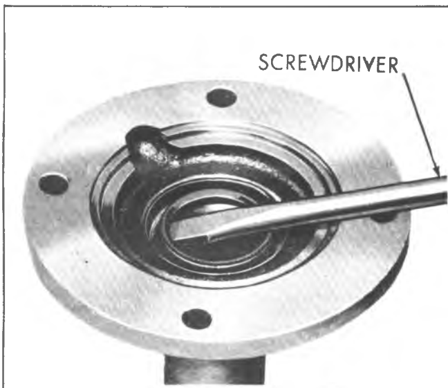
Fig. 7B-14J—Removing Bearing Retainer Oil Seal
