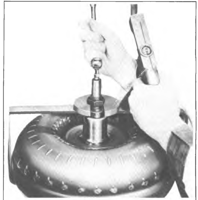
Fig. 7A-4B--Checking Converter for Leaks
