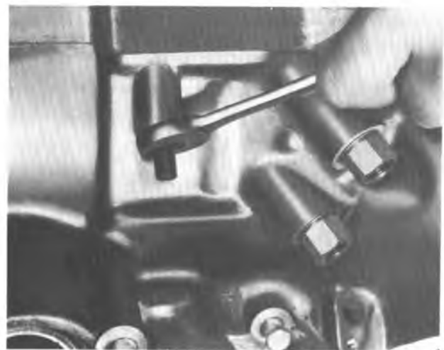
Figure 7A5-90 Intermediate Band Adjustment
