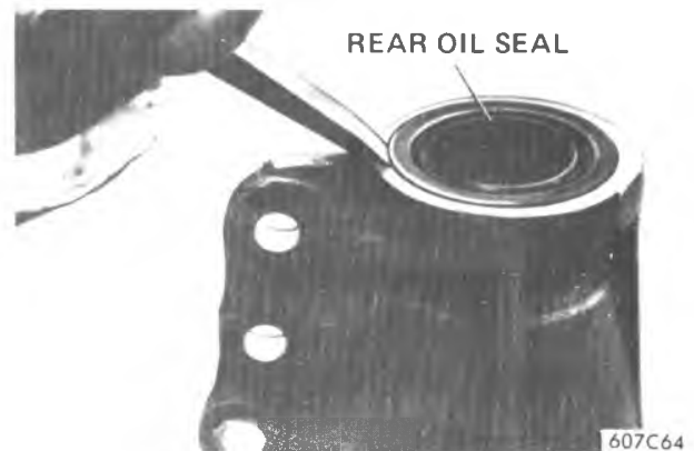
Figure 7A1-53 Removing Rear Oil Seal
