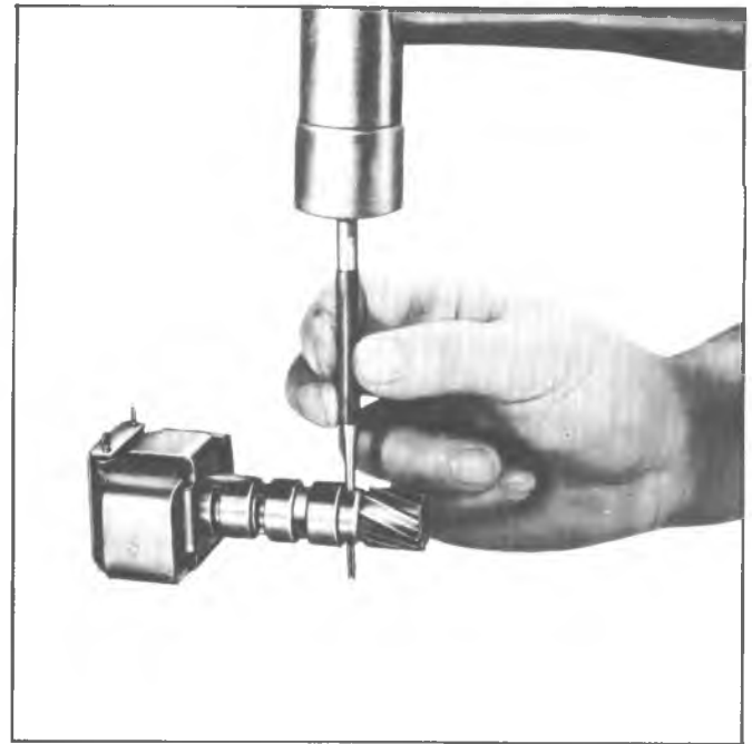
Fig. 7A-60C--Removing Governor Gear Retaining Pin
