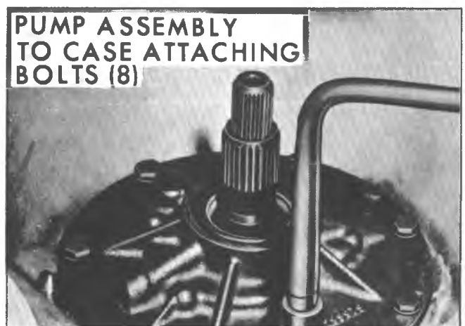
Fig. 7A-29B--Removing Pump Attaching Bolts
