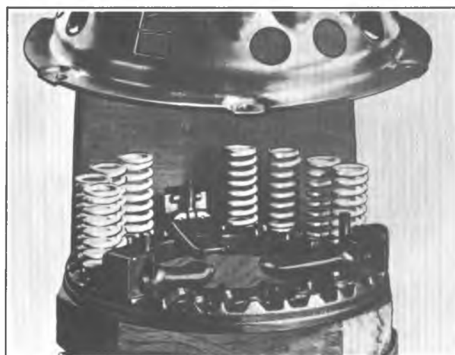
Fig. 7C-10E-Assembling Cover and Pressure Plate
