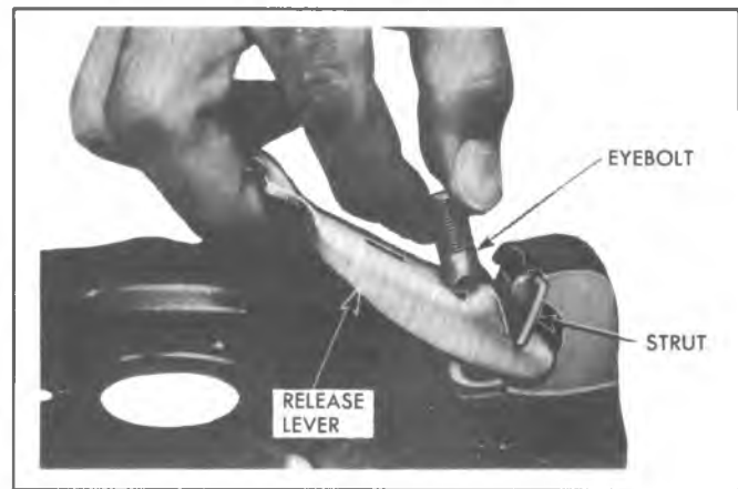
Fig. 7C-5E-Removing or Installing Lever
