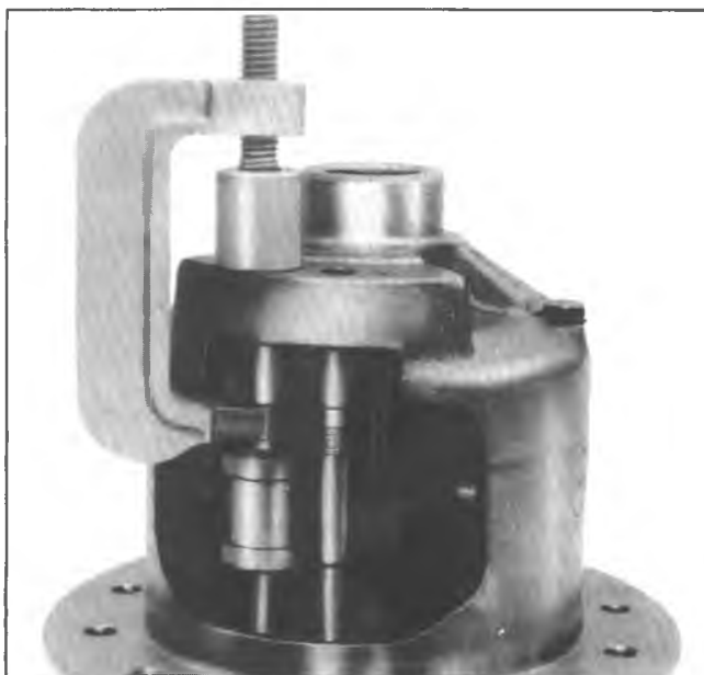
Fig. 4B-5H-Bearing Puller J-26252
