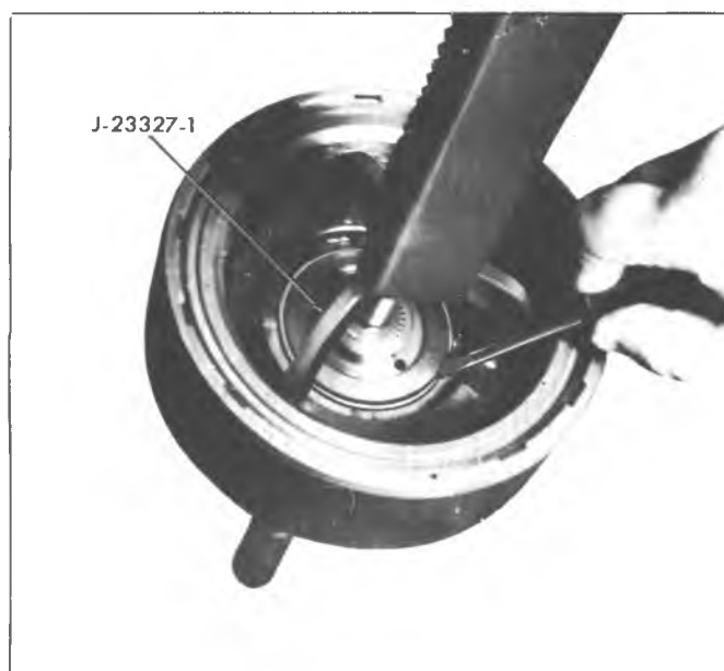
Fig. 7A-84B--Compressing Forward Clutch Piston Return Seat
