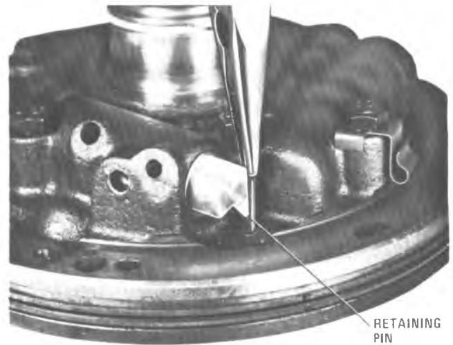
Figure 7A1-139C Removing Retaining Pin
