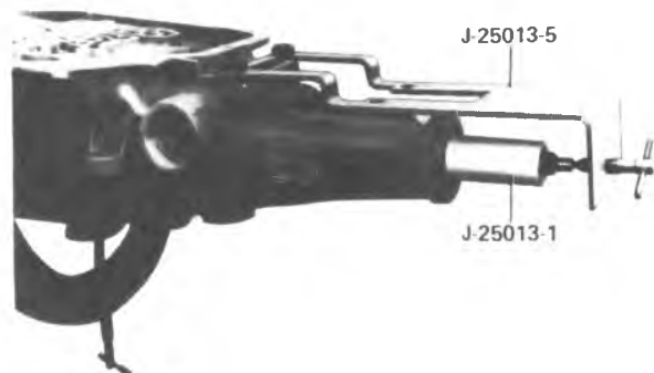
Figure 7A1-85 Installing Tools on Rear End of Case
