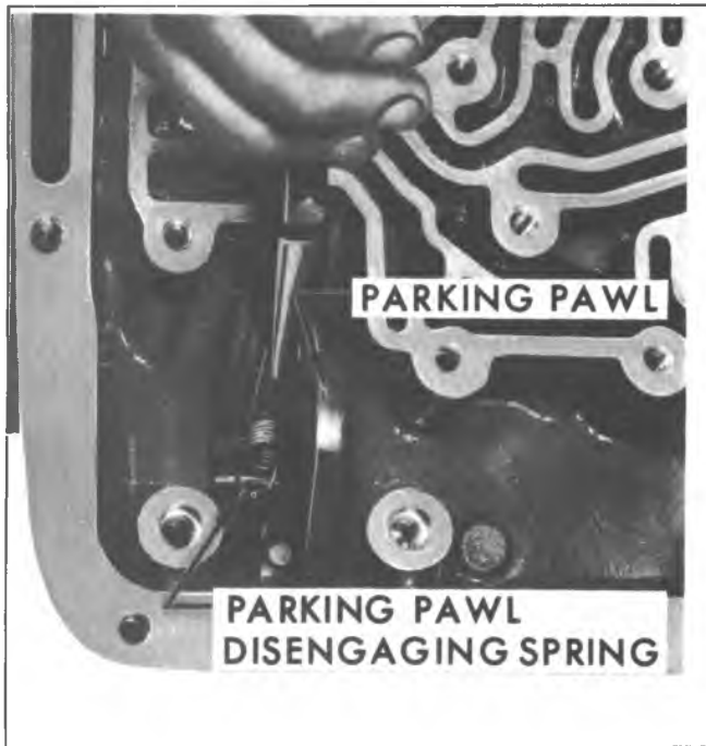
Fig. 7A-26B--Removing Parking Pawl Disengaging Spring
