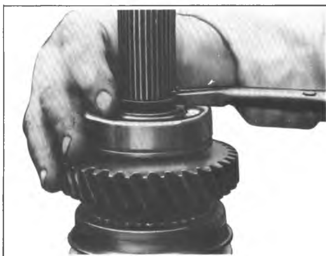
Fig. 7B-11K—Removing Rear Bearing Snap Ring
