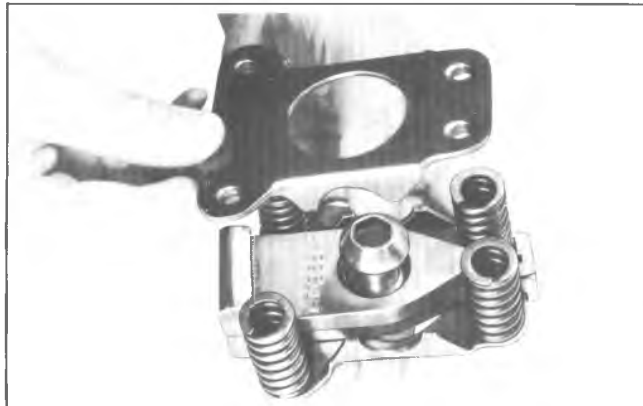
Fig. 12D--Installing Spring Pack Compression Tool (Corvette)
