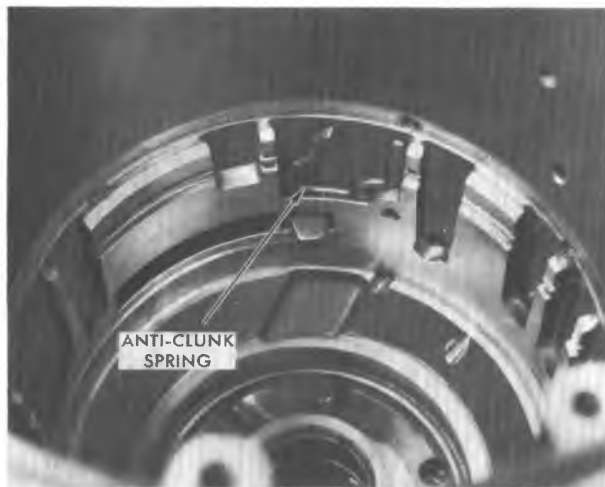
Figure 7A5-84 Anti Clunk Spring Piston
