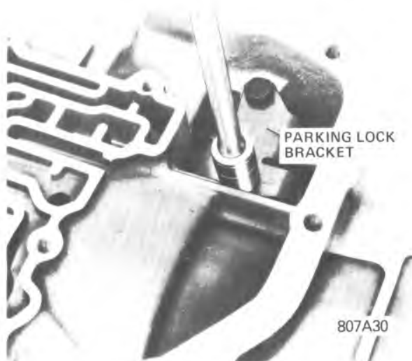
Figure 7A1-58 Removing Parking Pawl Bracket Bolt
