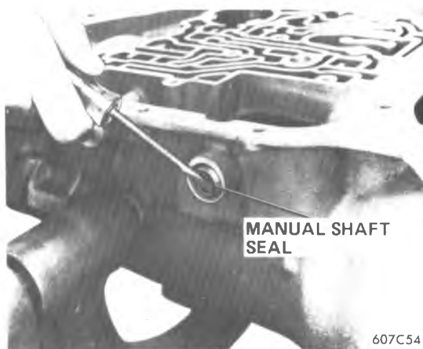
Figure 7A1-57 Removing Manual Shaft Seal From Case
