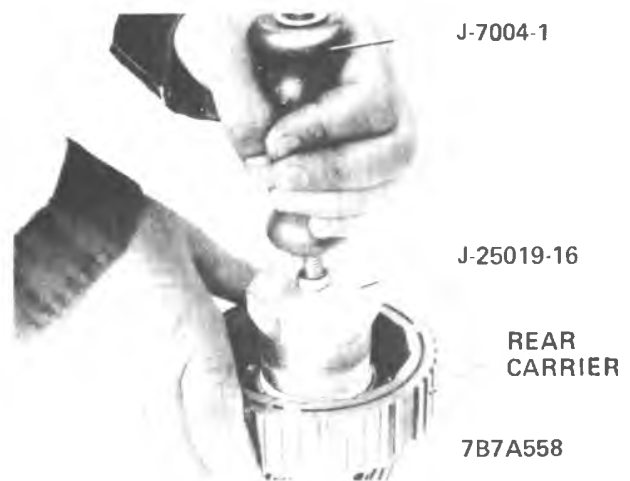
Figure 7A1-197 Removing Rear Carrier Bushing
