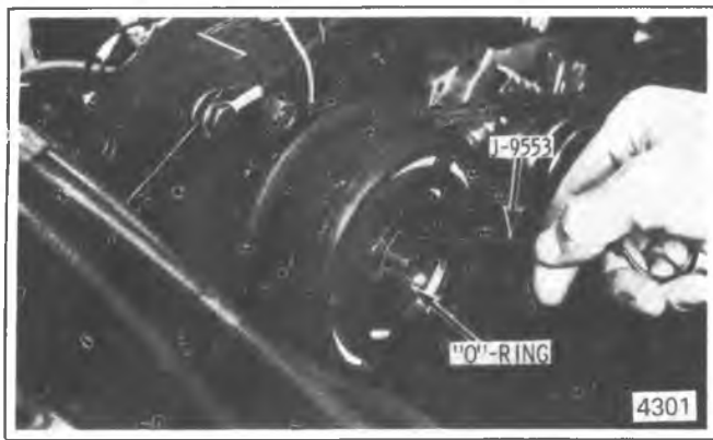
Figure 1D-95 Removing R-4 O-Ring (On Car)
