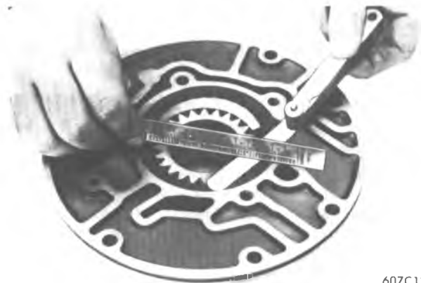
Figure 7A1-145 Checking Pump Body-to-Gear End Clearance
