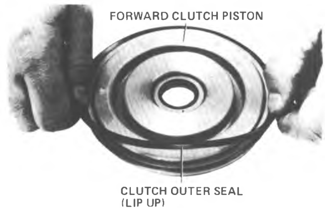
Figure 7A1-126 Removing or Installing Outer Piston Seal
