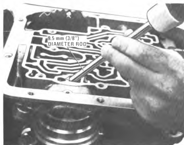
Figure 7A1-29C Installing 3rd Accumulator Check Valve Assy.
