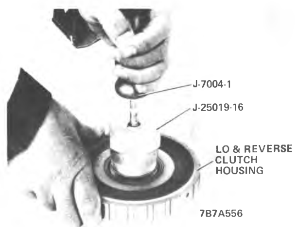
Figure 7A1-195 Removing Lo and Reverse Clutch Housing Bushing
