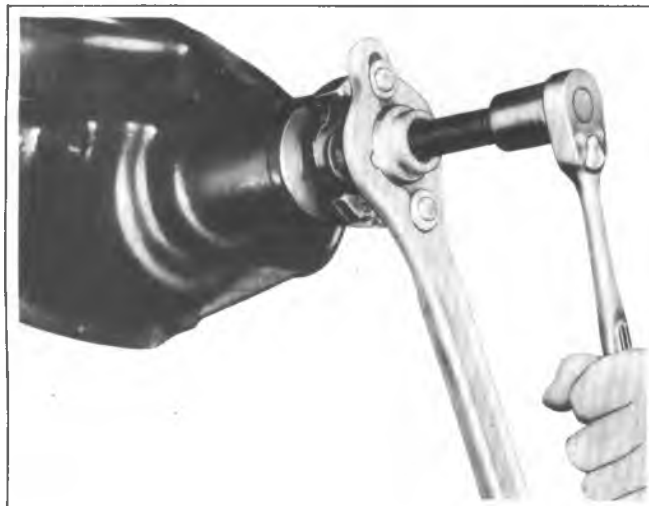
Fig. 13B--Drive Pinion Flange Removal
