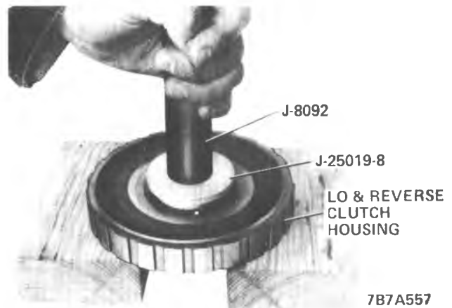
Figure 7A1-196 Installing Lo and Reverse Clutch Housing Bushing
