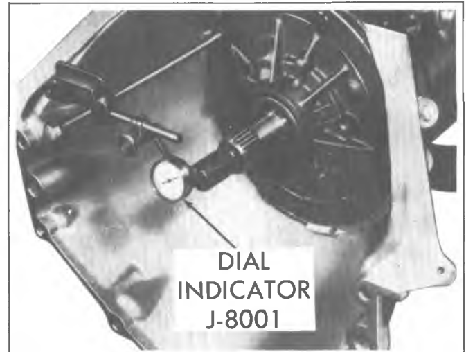
Fig. 7A-29C--Checking Front Unit End Play
