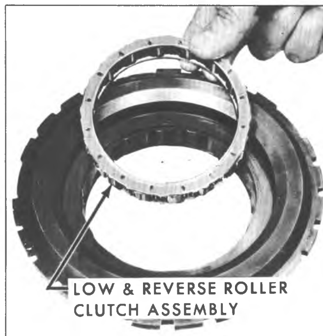
Fig. 7A-96B--Removing Overrun Roller Clutch Assembly
