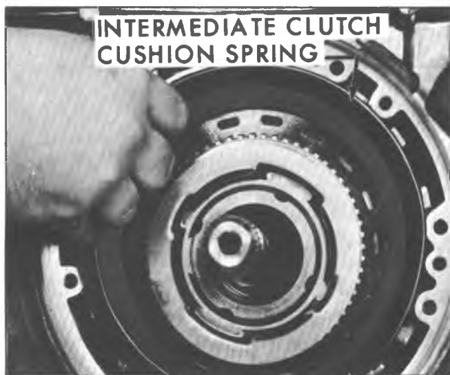
Fig. 7A-31B--Removing Intermediate Clutch Cushion Spring
