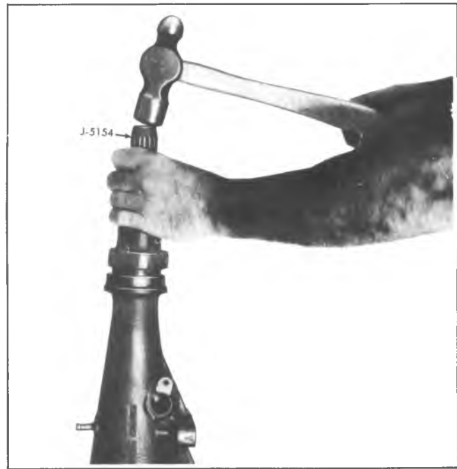
Fig. 7B-16B—Installing Extension Housing Seal
