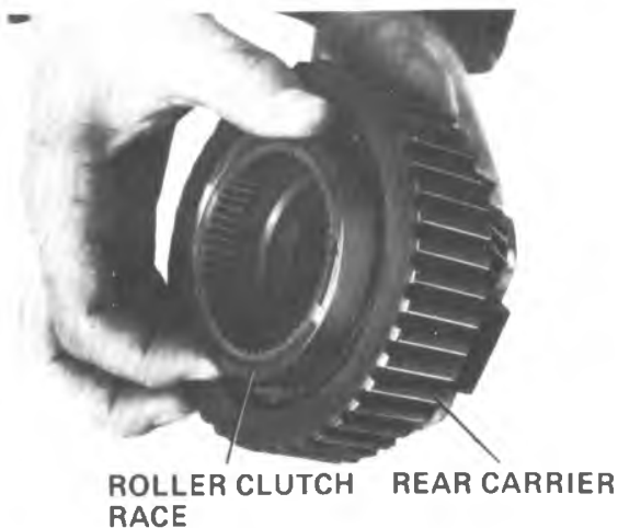
Figure 7A1-82 Installing Roller Clutch Race
