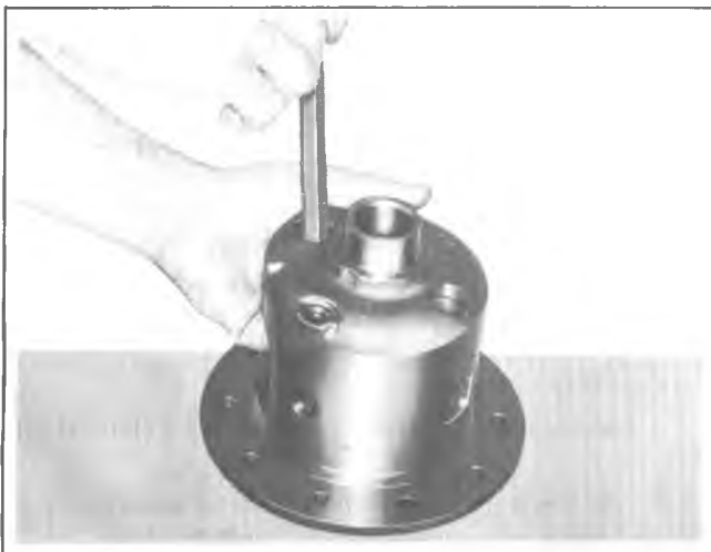
Fig. 8D-Removing Side Gear
