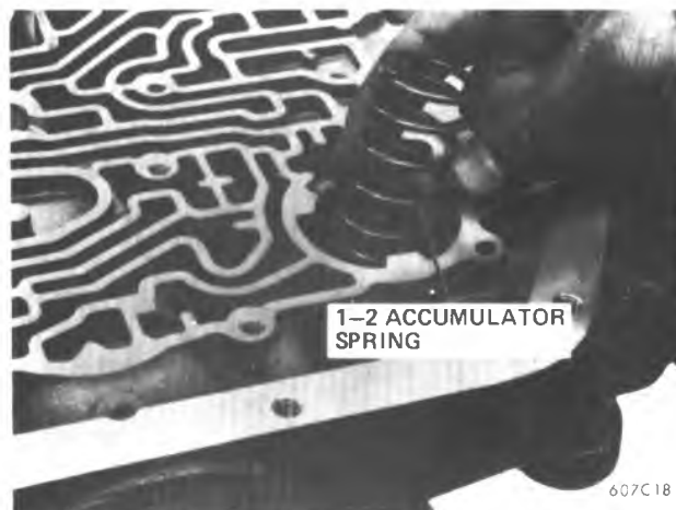
Figure 7A1-172 Installing 1-2 Accumulator Spring
