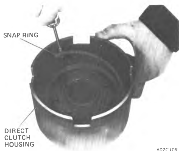
Figure 7A1-113 Removing Direct Clutch Snap Ring
