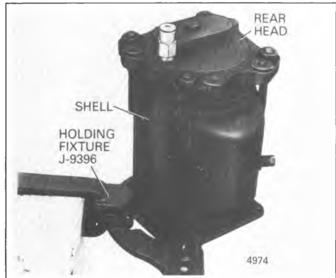
Figure 1D-29 A-6 Compressor Installed in Holding Fixture
