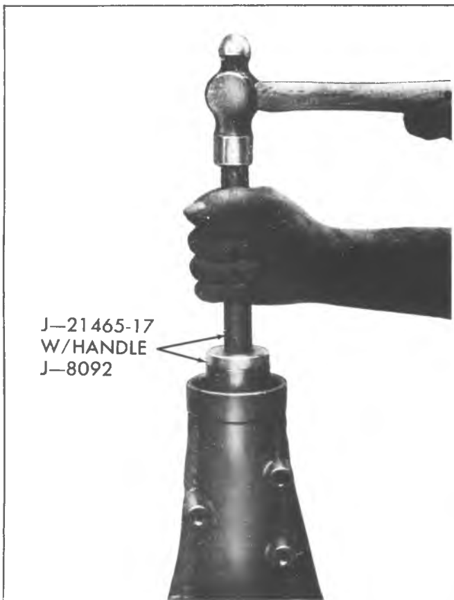
Fig. 7B-14K-Removing Rear Extension Bushing
