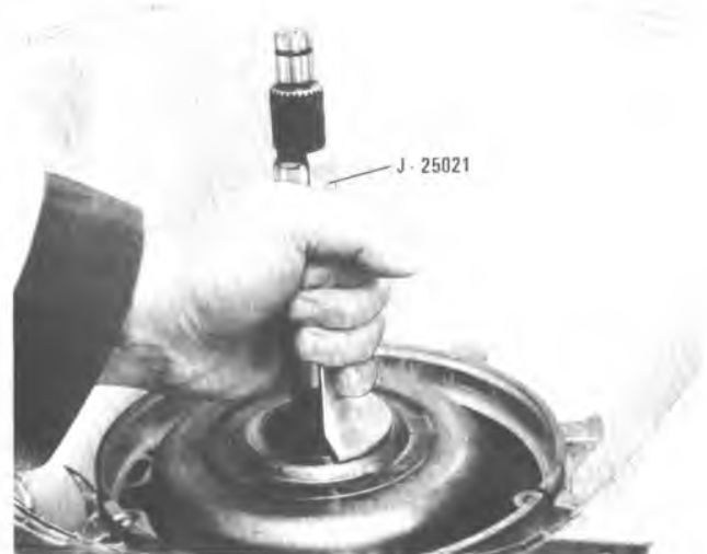
Figure 7A1-135 Installing Direct and Forward Clutch Assemblies
