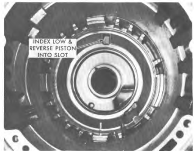
Figure 7A5-80 Low & Reverse Piston Indexing Slot
