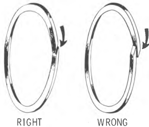
Figure 7A1-16 Teflon Oil Seal Rings
