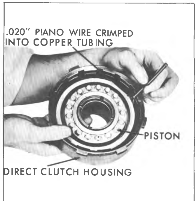
Fig. 7A-78B--Installing Direct Clutch Piston
