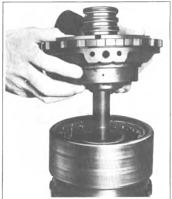
Fig. 7A-46C--Removing Center Support Assembly
