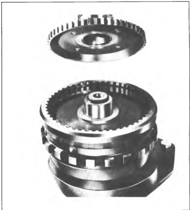
Fig. 7A-145C--Installing Output Shaft
