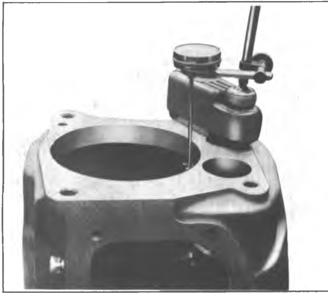
Fig. 7B-20K—Checking Countergear End Play
