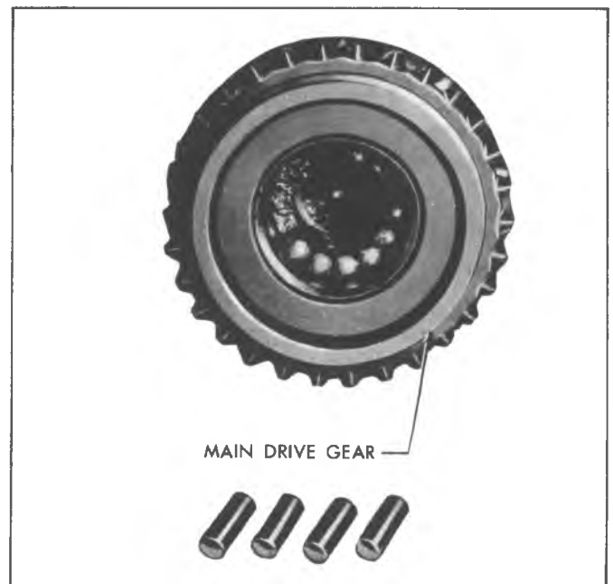
Fig. 7B-17A--Loading Pilot Bearings
