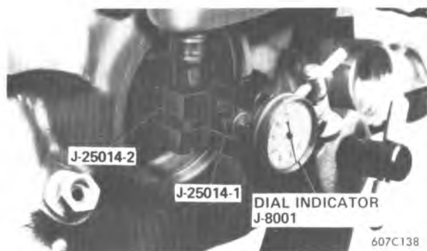
Figure 7A1-160 Intermediate Band Apply Gages
