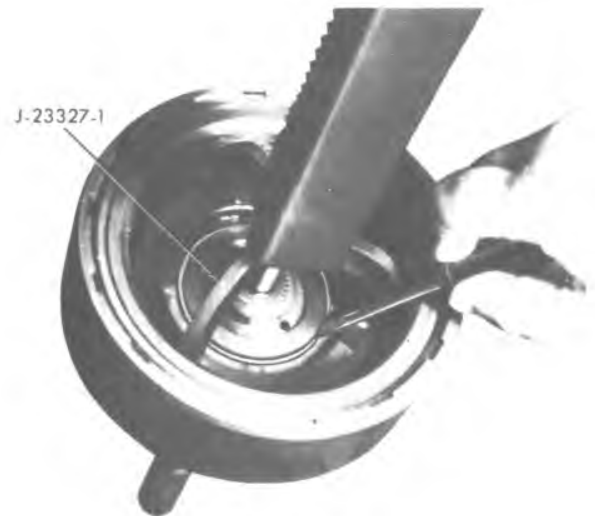
Figure 7A5-64 Compressing Forward Clutch Spring Retaining Seat
