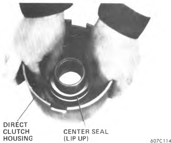
Figure 7A1-117 Removing Center Seal From Direct Clutch Housing
