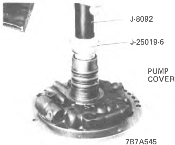
Figure 7A1-184 Installing Pump Cover Bushing - Rear
