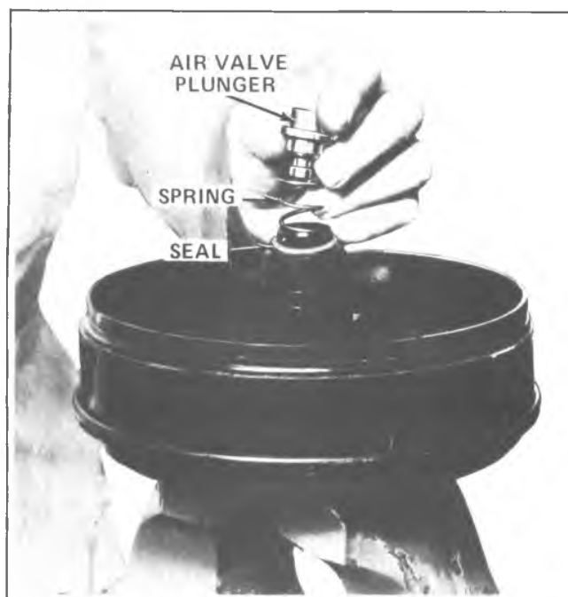
Fig. 5-10B—Installing Air Valve Plunger
