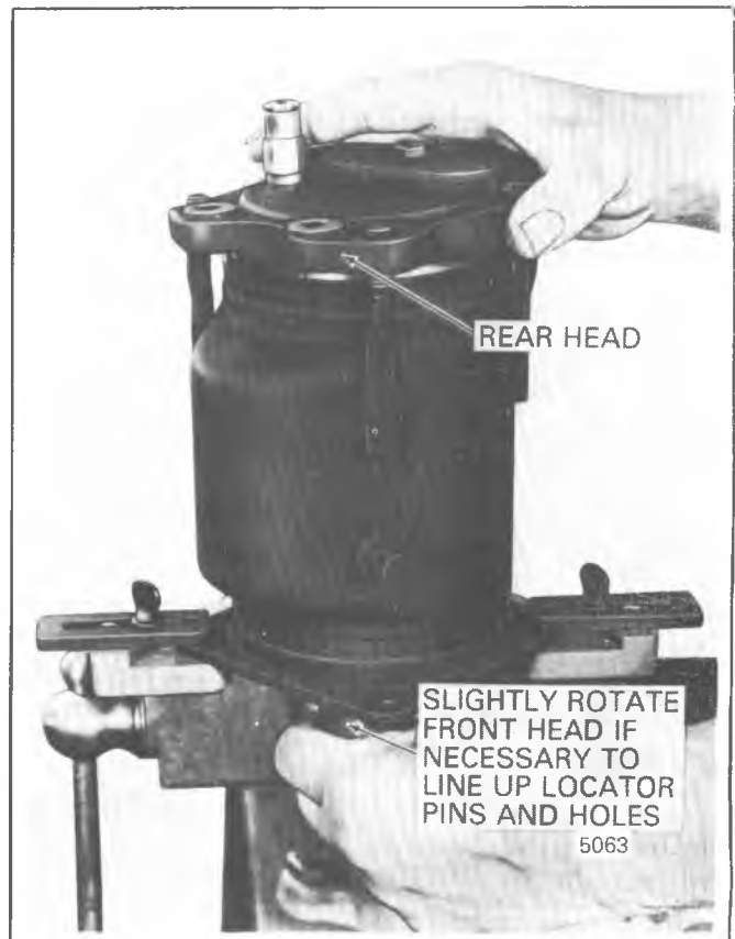
Figure 1D-72 Installing A-6 Rear Head
