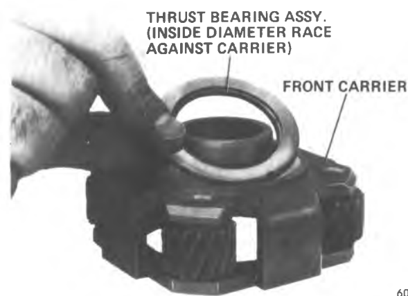
Figure 7A1-105 Installing Thrust Bearing Assembly Onto Front Carrier
