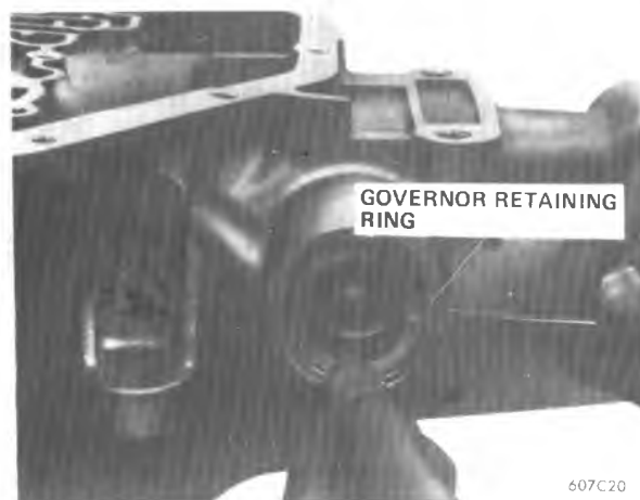
Figure 7A1-23 Removing Governor Cover Retaining Ring
