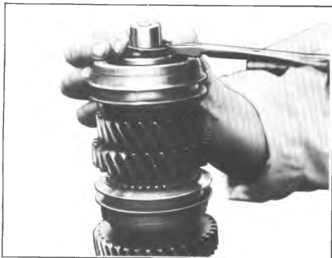
Fig. 7B-9K—Removing 3-4 Clutch Assembly Retainer
