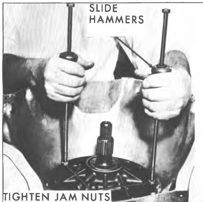
Fig. 7A-30B--Removing Pump from Case
