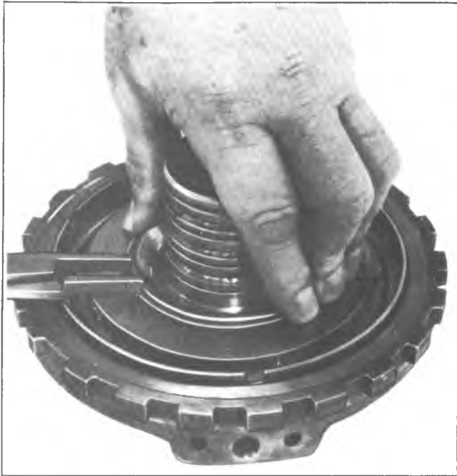
Fig. 7A-113C--Removing Intermediate Clutch Piston Snap Ring
