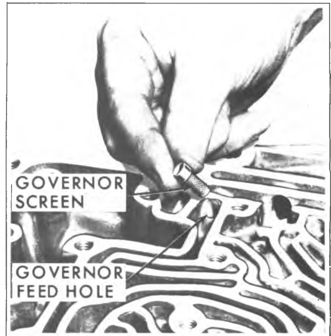
Fig. 7A-20B--Removing Governor Feed Screen
