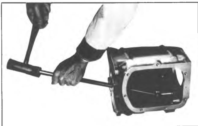
Fig. 7B-6A—Removing Reverse Idler Shaft
