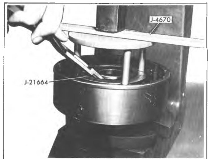
Fig. 7A-94C--Removing or Installing Direct Clutch Snap Ring
