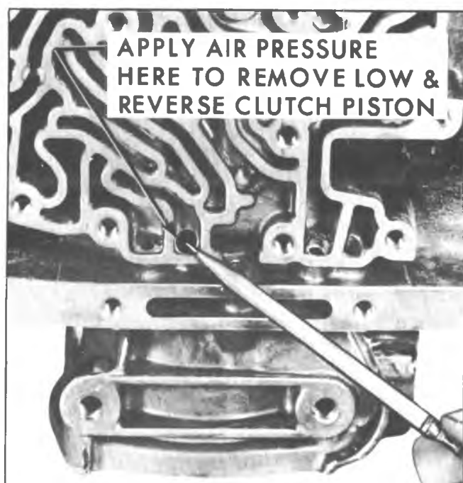
Fig. 7A-50B--Removing Low and Reverse Clutch Piston
