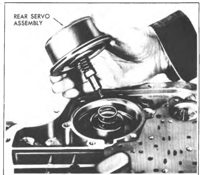
Fig. 7A-181C--Installing Rear Servo Assembly
