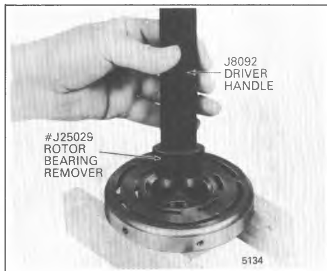
Figure 1D-84 R-4 Clutch Rotor Bearing Removal
