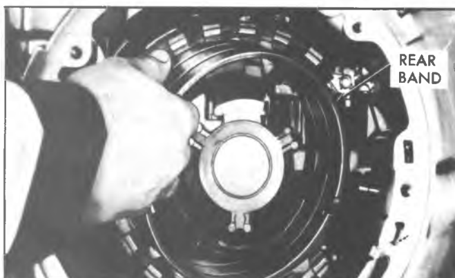
Fig. 7A-156C--Installing Rear Band
