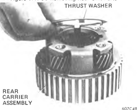
Figure 7A1-51 Removing Thrust Washer
