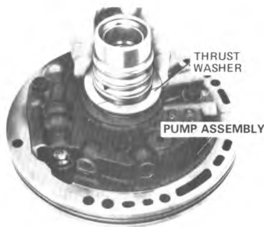
Figure 7A1-138 Removing Thrust Washer from Pump
