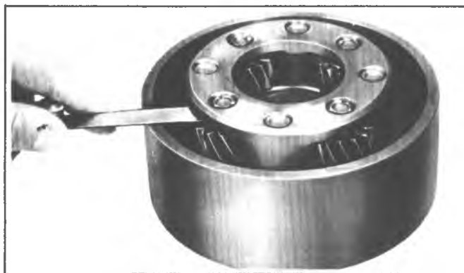
Fig. 7A-128C--Checking Pinions End Play
