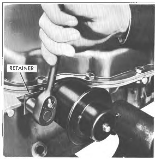
Fig. 7A-3C--Removing Modulator Retainer
