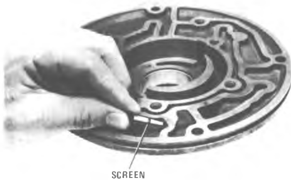
Figure 7A1-141B Removing Screen
