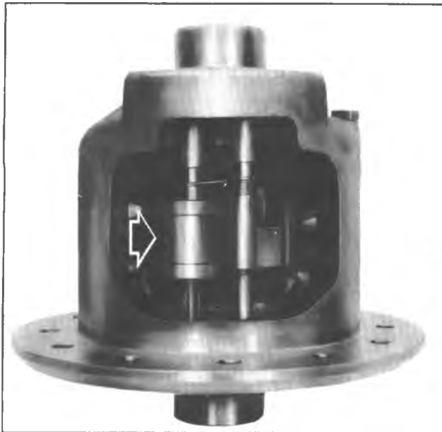
Fig. 4B-4H-Governor and Latching Bracket
