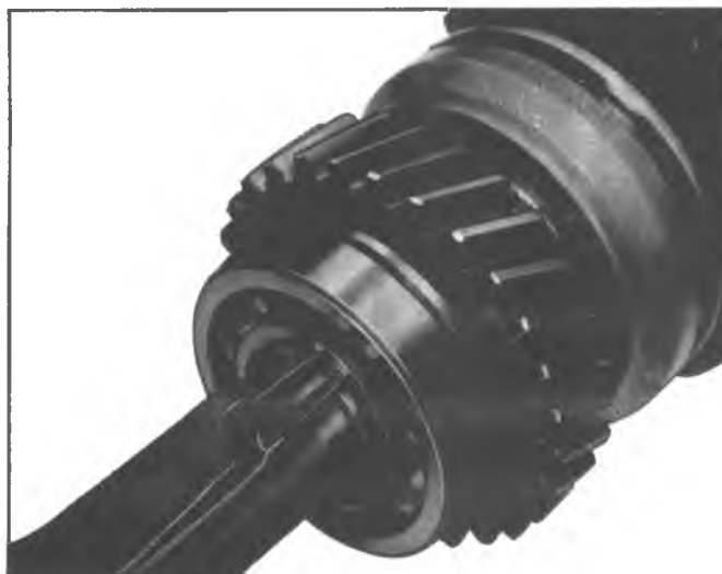
Fig. 7B-8A—Removing Rear Bearing Retaining Ring
