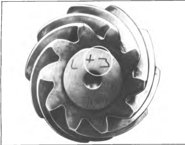
Fig. 20F—Marking From Nominal on Pinion
