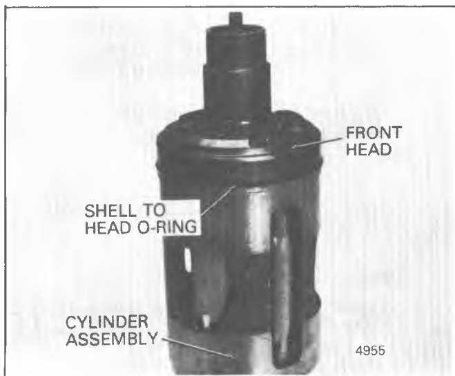
Figure 1D-71 A-6 Shell-To-Front Head O-Ring Installation
