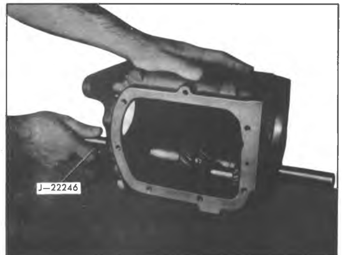
Fig. 7B-5A--Removing Counter Gear Shaft
