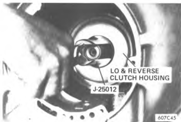
Figure 7A1-97 Installing Low and Reverse Clutch
