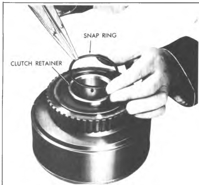
Fig. 7A-92C--Removing Intermediate Clutch Retainer Snap Ring
