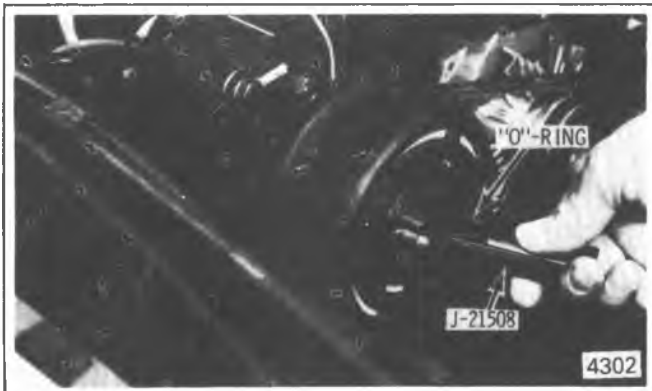
Figure 1D-96 Installing R-4 O-Ring (On Car)
