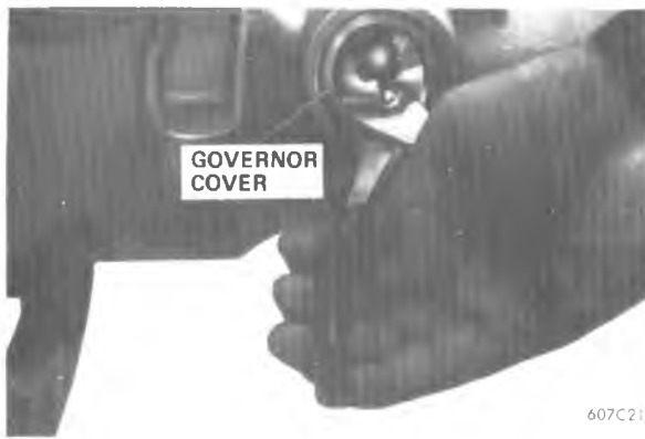
Figure 7A1-24 Removing Governor Cover
