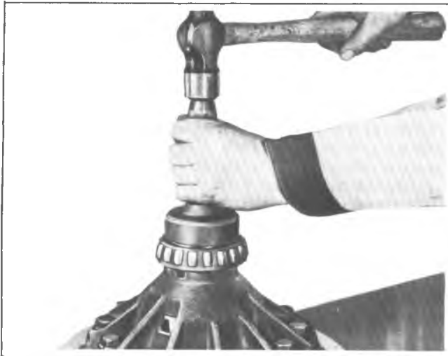
Fig. 8G--Differential Bearing Installation
