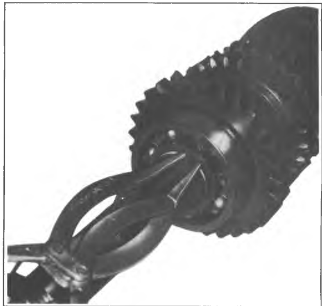
Fig. 7B-8J—Rear Bearing to Mainshaft Snap Ring
