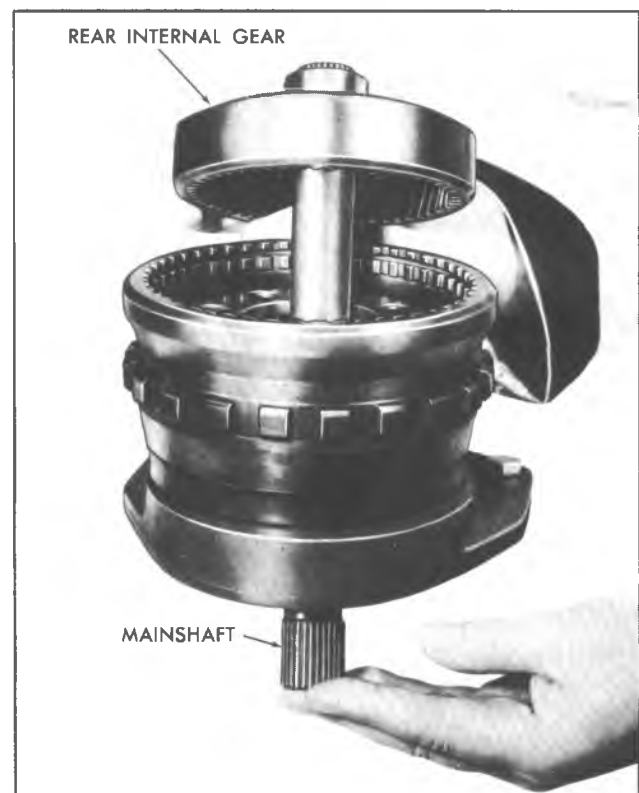
Fig. 7A-51C--Removing Rear Internal Gear and Mainshaft
