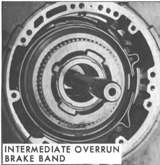
Fig. 7A-34B--Removing Intermediate Overrun Brake Band
