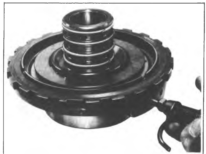
Fig. 7A-126C--Air Checking Intermediate Clutch Piston
