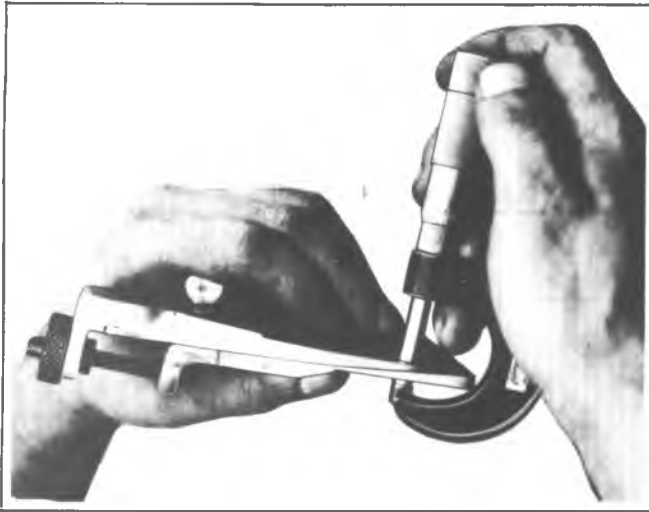
Fig. 8B--Measuring Gage Plate Thickness
