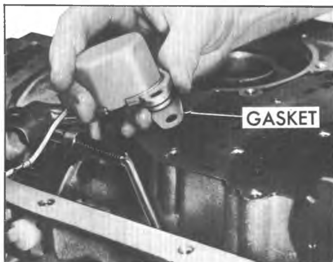
Fig. 7A-18C--Removing Detent Solenoid and Gasket
