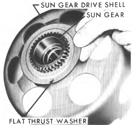
Figure 7A5-71 Removing Sun Gear to Drive Shell
