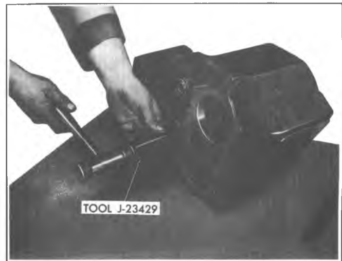
Fig. 7E-8R-Removing Idler Gear Shaft
