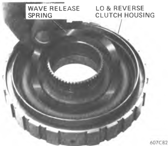
Figure 7A1-89 Removing Lo and Reverse Clutch Wave Release Spring.
