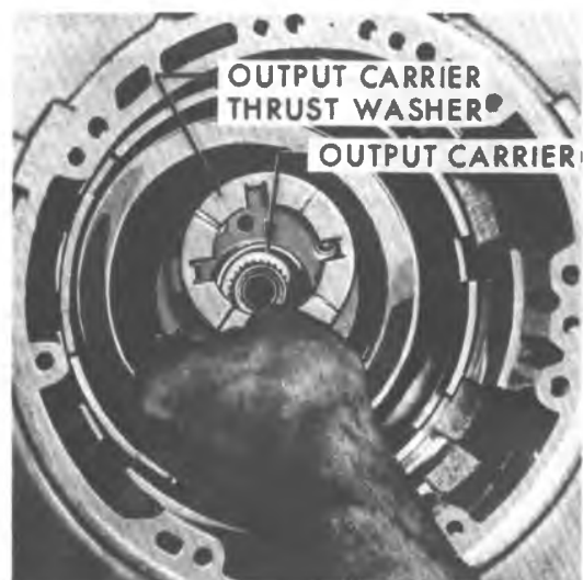
Figure 7A5-29 Output Carrier and Thrust Washer Removal
