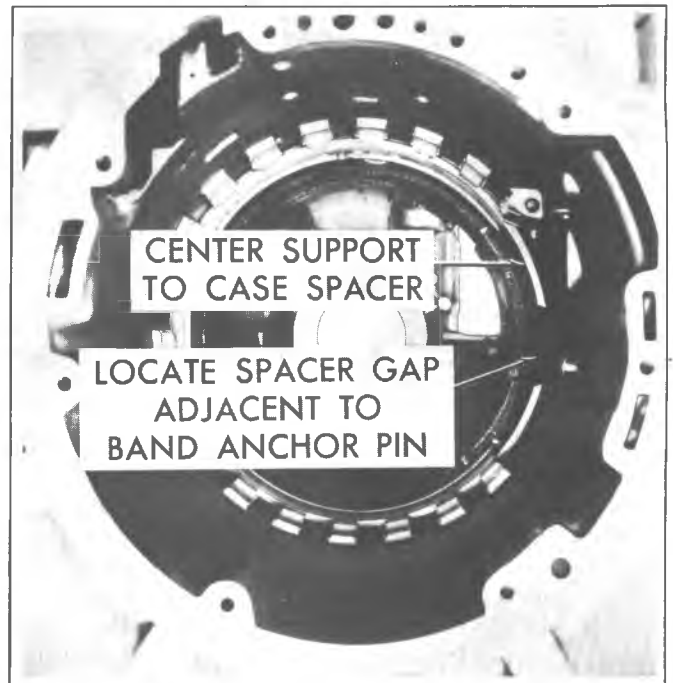
Fig. 7A-157C--Installing Center Support to Case Spacer
