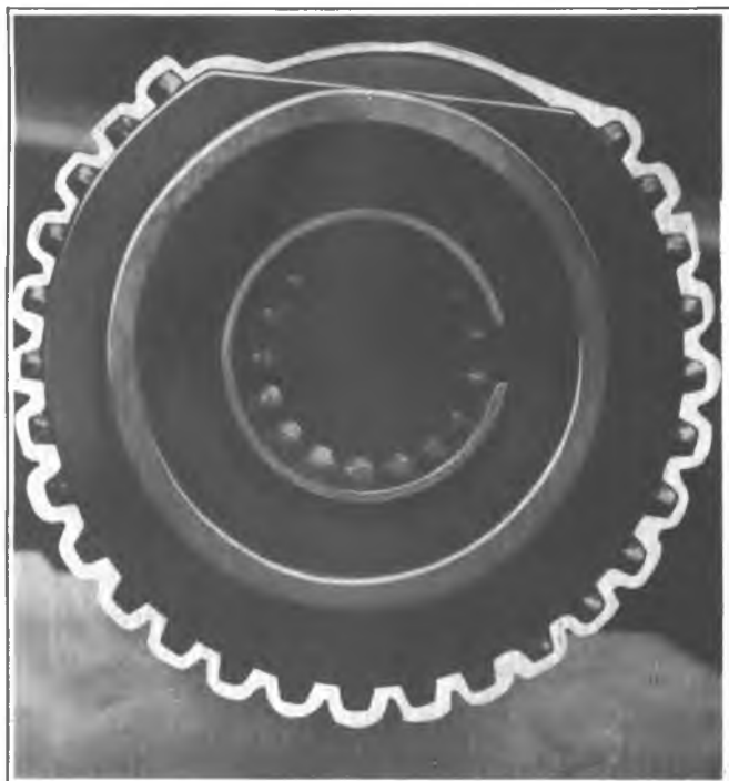
Fig. 7B-12L-Pilot Roller Bearing Installed
