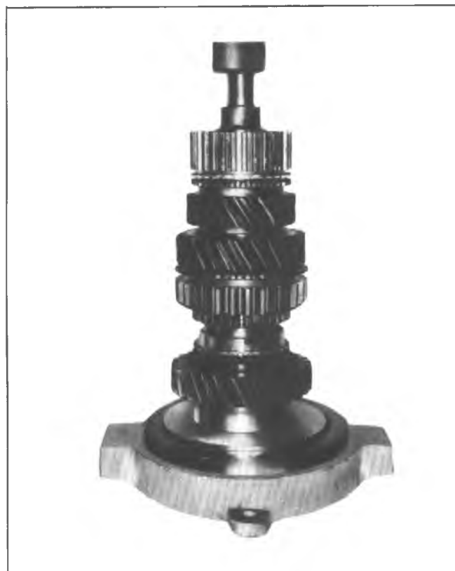
Fig. 7B-17J-Installing Rear Bearing
