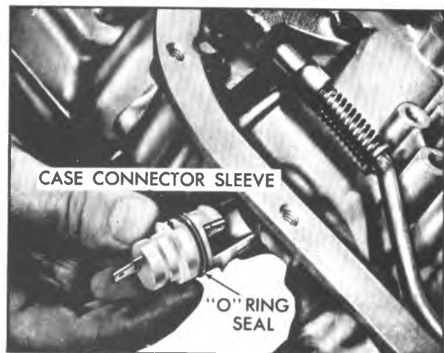
Fig. 7A-178C--Installing Electrical Connector and "O" Ring Seal
