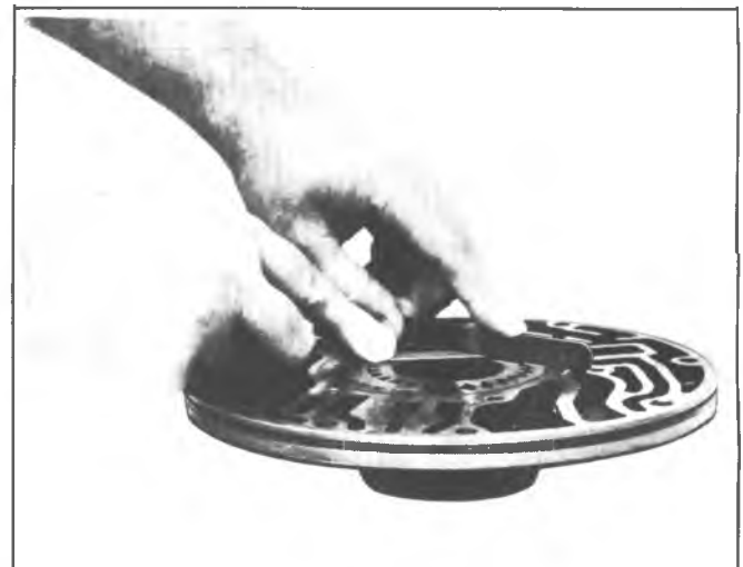
Fig. 7A-63B--Checking Pump Body to Gear Face Clearance
