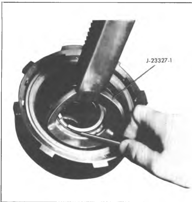
Fig. 7A-76B--Removing Direct Clutch Outer and Inner Seals
