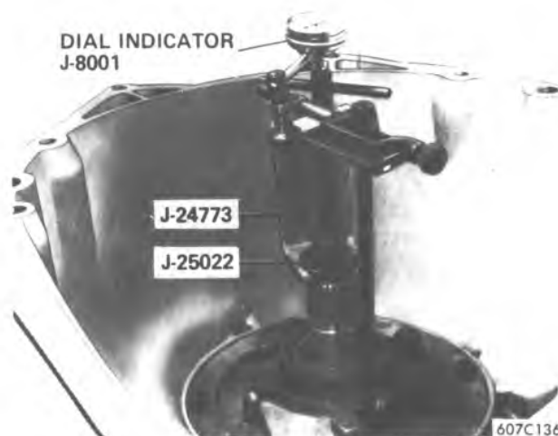
Figure 7A1-153 Checking Front Unit End Play
