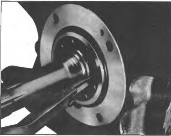
Fig. 7B-2A--Removing Clutch Gear Bearing Retaining Ring
