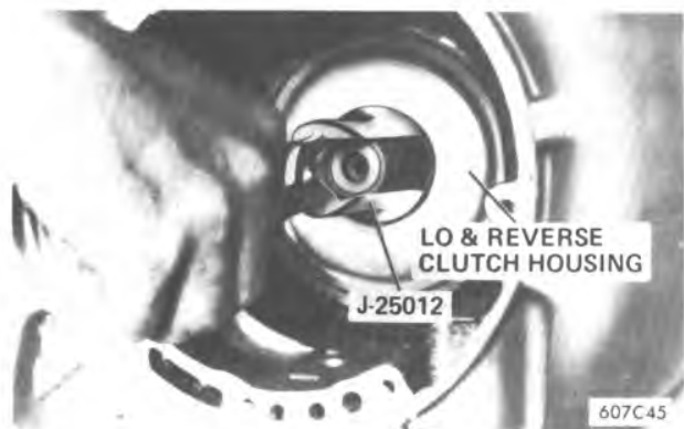
Figure 7A1-48 Removing Low and Reverse Clutch Housing
