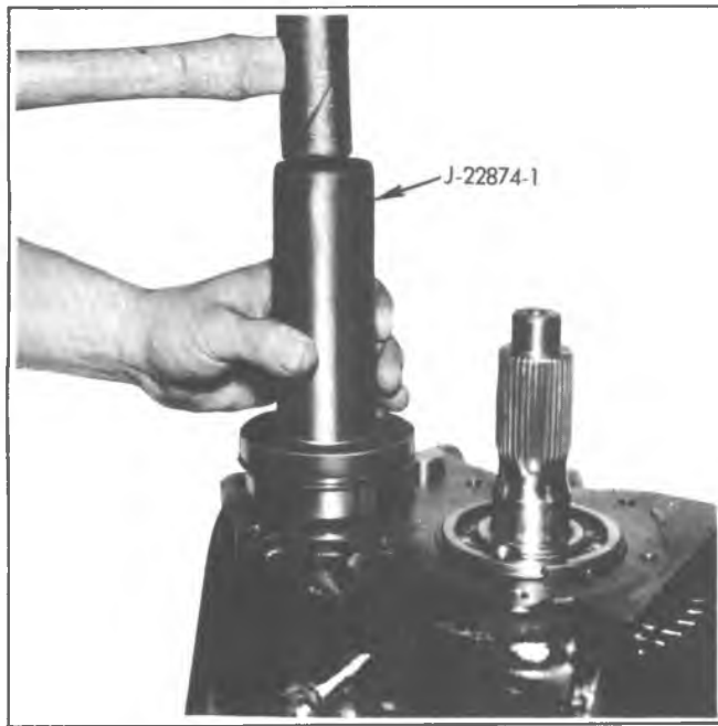
Fig. 7B-25L—Installing Countergear Rear Bearing
