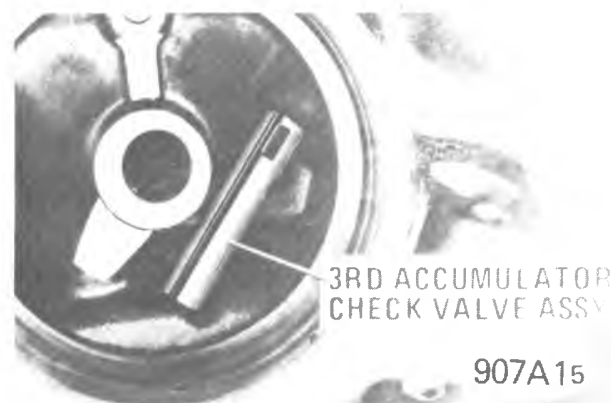
Figure 7A1-29A 3rd Accumulator Check Valve Assembly
