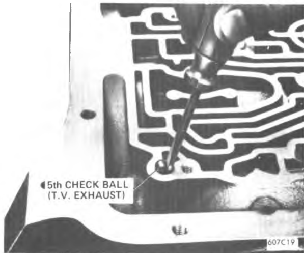
Figure 7A1-173 Installing 5th Check Ball
