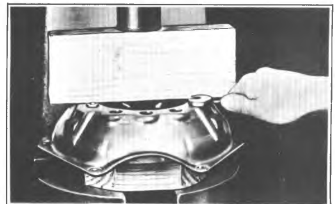
Fig. 7C-2E-Compressing Clutch
