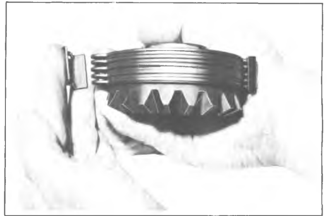
Fig. 9D-Assembling Clutch Pack
