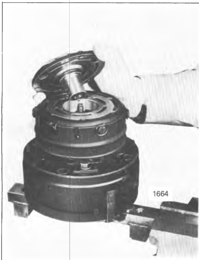
Figure 1D-79 Installing R-4 Shaft Key
