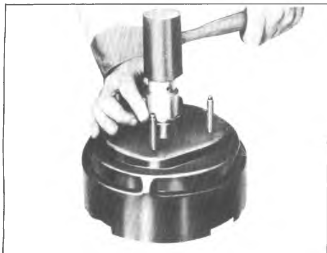
Fig. 5-6B—Removing Rear Seal
