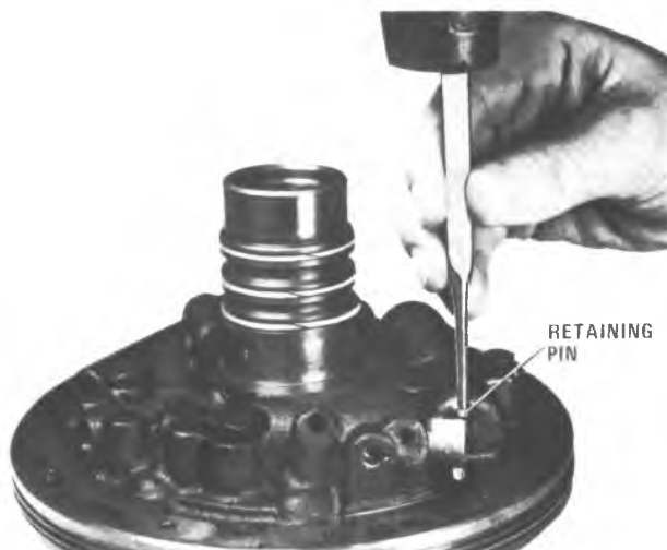
Figure 7A1-150B Install Retaining Pin
