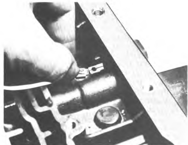
Figure 7A1-164B Installing Lead Wire
