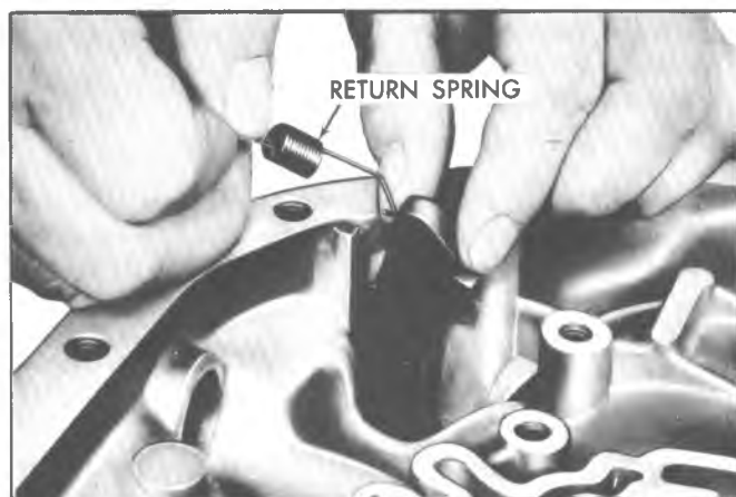
Fig. 7A-24C--Removing Parking Pawl Return Spring
