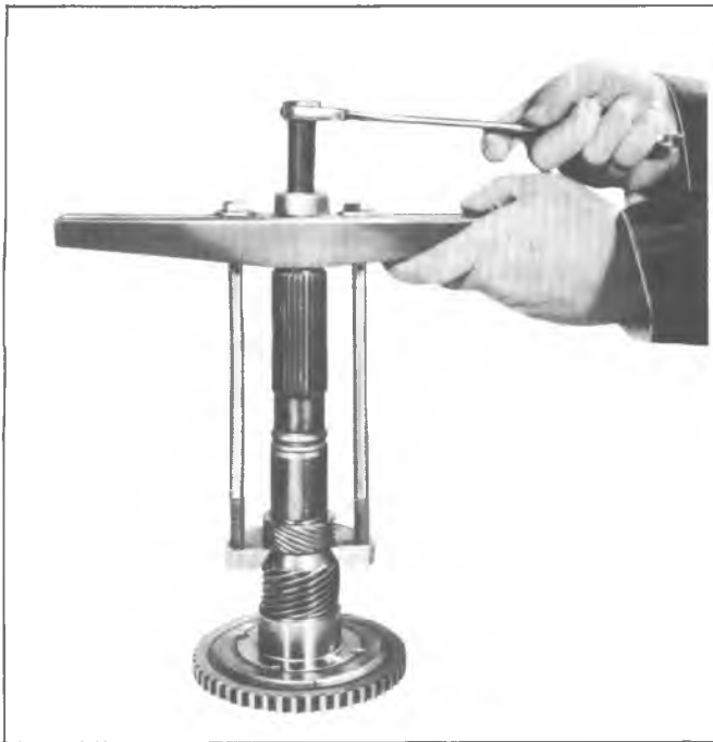
Fig. 7A-55C--Removing Steel Speedometer Drive Gear
