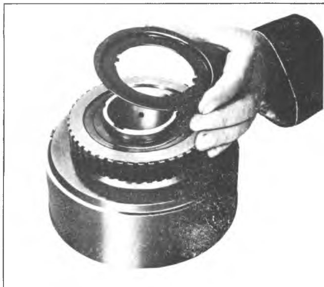
Fig. 7A-109C--Installing Intermediate Clutch Retainer
