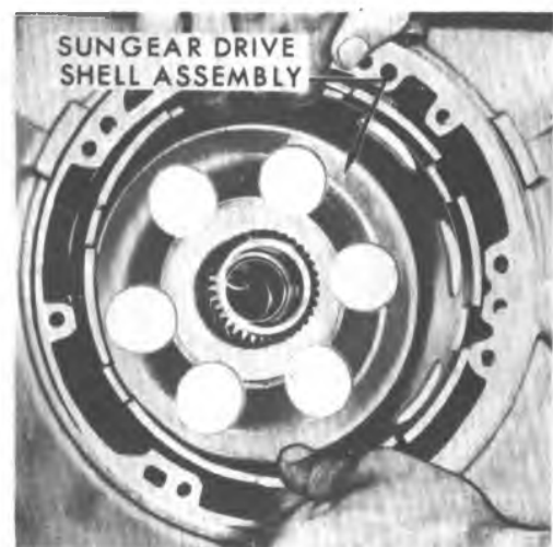
Figure 7A5-30 Sun Gear Drive Shell Removal
