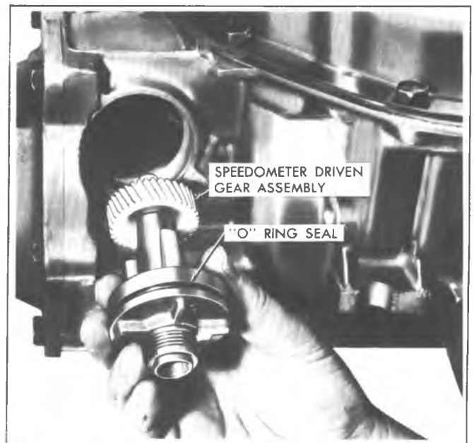
Fig. 7A-188C--Installing Speedometer Driven Gear and Sleeve
