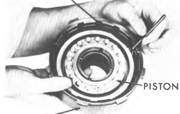
Figure 7A5-58 Installing Direct Clutch Piston
