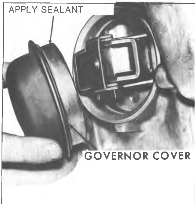
Fig. 7A-10B--Governor Cover and "O" Ring Seal
