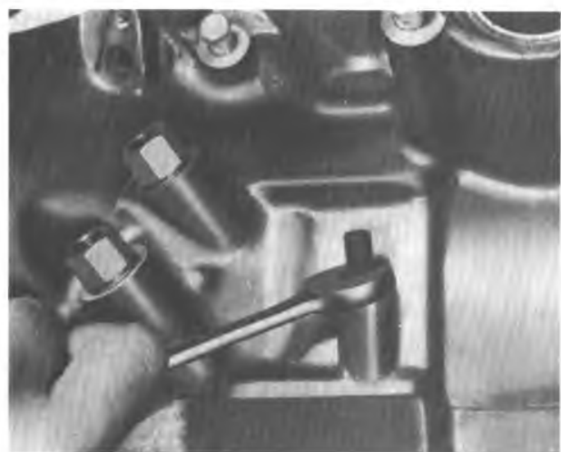
Figure 7A5-24 Intermediate Band Anchor Bolt
