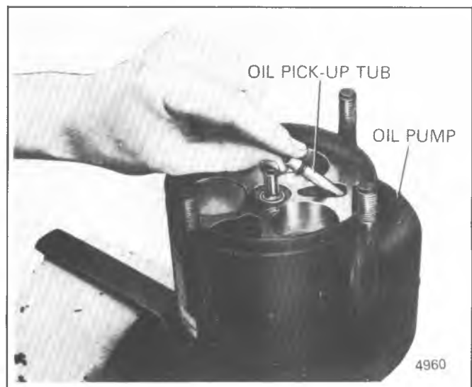
Figure 1D-69 Installing A-6 Oil Pick-up Tube
