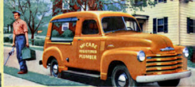
MODEL 3107 CANOPY EXPRESS 116" W.B., MAX. G.V.W. 4800 LB. Over-all dimensions are similar to those of 3105, Panel
