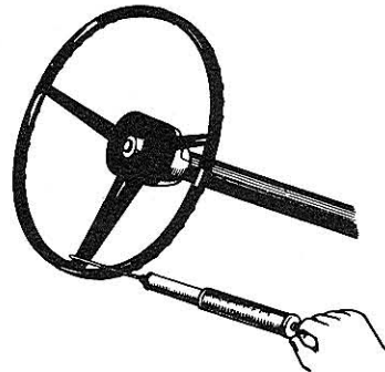
Fig.6-37 Worm Bearing Preload Adjustment
