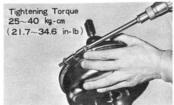
Fig.6-69 Tightening Brake Band
