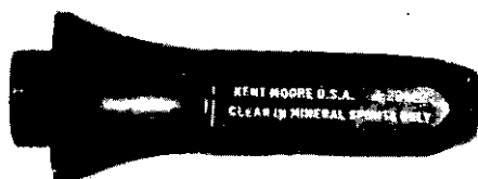
J-22922 TRANSMISSION CASE EXTENSION HOUSING SEAL INSTALLER
