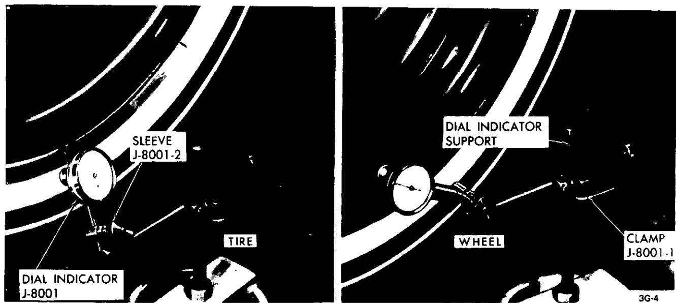
Figure 3G-4 Checking Lateral Runout
