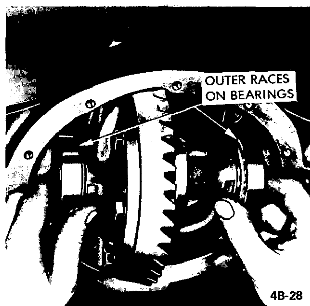
Figure 4B-28 Installing Differential Case Assembly
