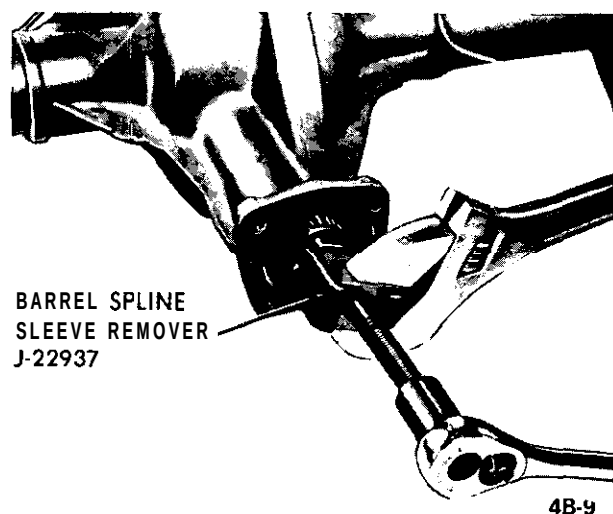
Figure 4B-9 Removing Barrel Spline Sleeve
