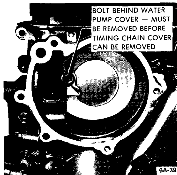
Figure 6A-39 Bolt Behind Water Pump
