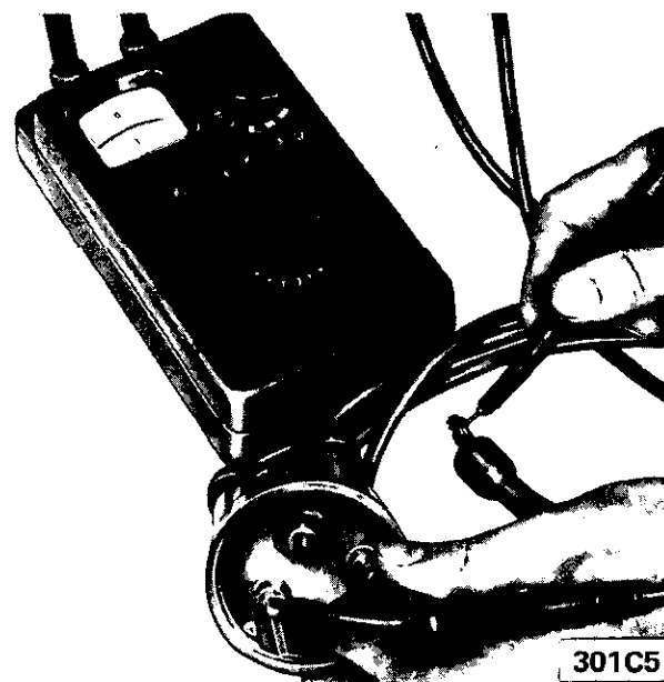
Figure 1C-5 Checking Ignition Wire Resistance
