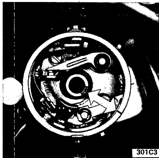
Figure 1C-3 Rotor Position for Firing No. 1 Cylinder
