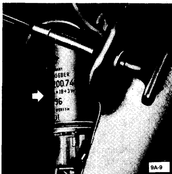
Figure 9A-9 Directional Flasher Unit
