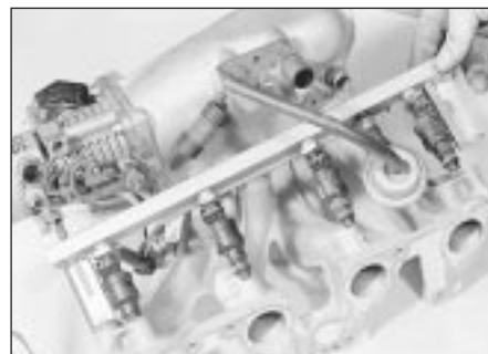
28.6C . . . and lift the fuel rail from the inlet manifold (inlet manifold removed for clarity) - SOHC model
