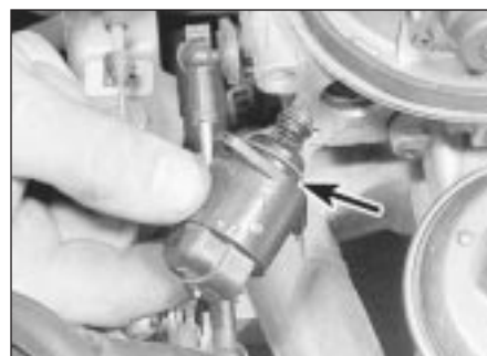
33.4B . . . to remove the stepper motor - renew sealing ring (arrowed)
