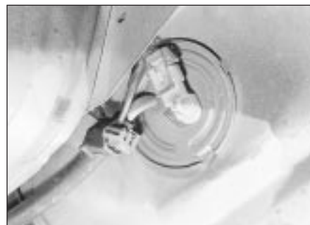
17.1 Fuel level sender unit - models with semi-independent rear axles
