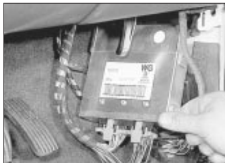
35.3 Withdrawing the fuel injection/ignition system ECU
