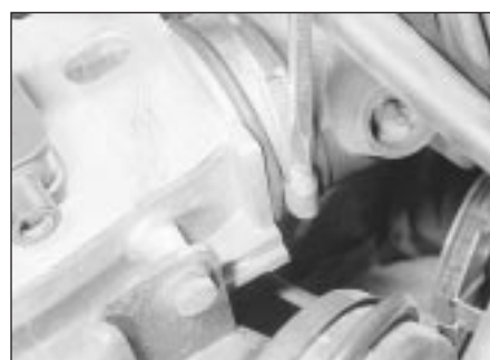
4.2 Loosening the air trunking clamp screw at the airflow meter
