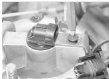
29.5 Unscrewing the injector retainer Torx screw
