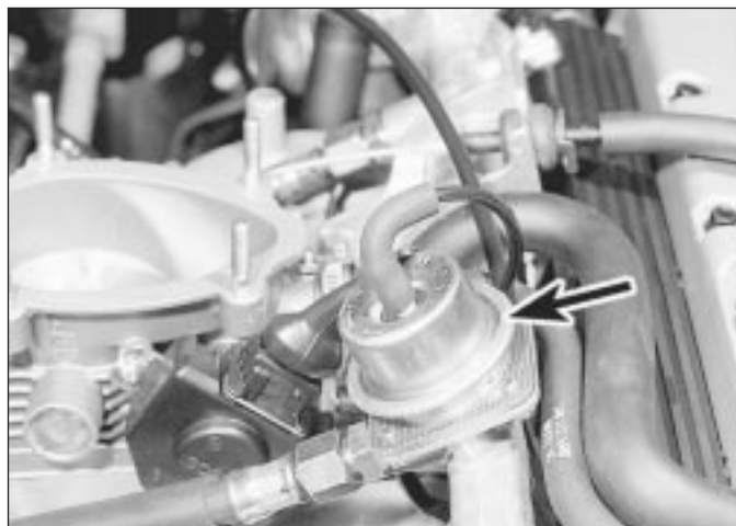
21.17 Fuel pressure regulator (arrowed) - DOHC model
