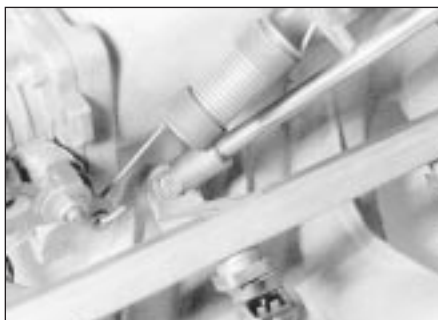
28.6B . . . and inner fuel rail securing bolts . . .
