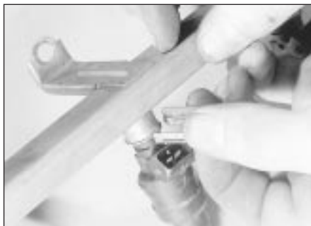
28.7A Withdraw the securing clip . . .
