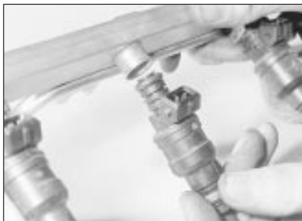
28.7B . . . then pull the injector from the fuel rail - SOHC model
