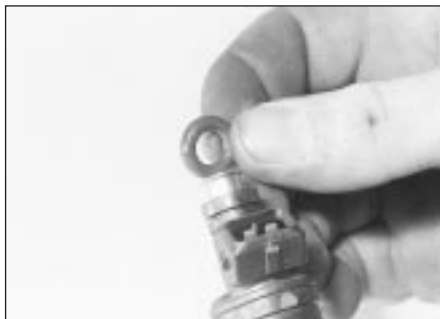
28.9 Fit new seals to the injectors
