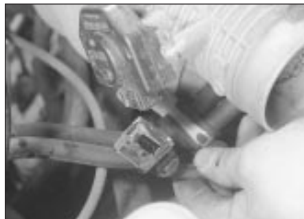
23.2 Disconnecting the throttle position sensor wiring plug - early SOHC models
