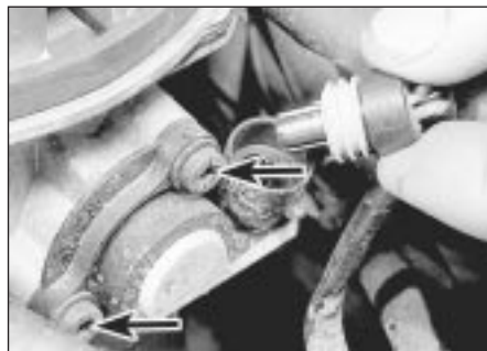
34.2 Disconnecting the throttle potentiometer wiring plug - note the mounting screws (arrowed)
