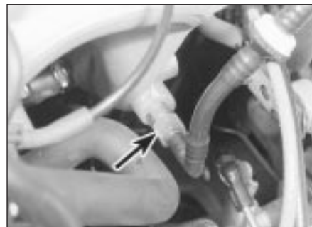
40.13 Brake servo vacuum hose connection at inlet manifold (arrowed) - DOHC models
