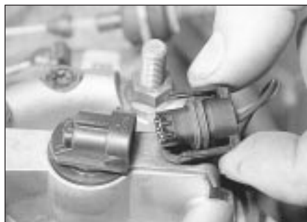
29.4 Disconnecting the fuel injector wiring plug - Multec systems
