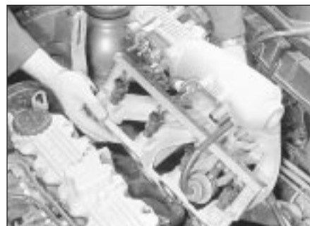
38.14B ...and withdraw the inlet manifold - SOHC models
