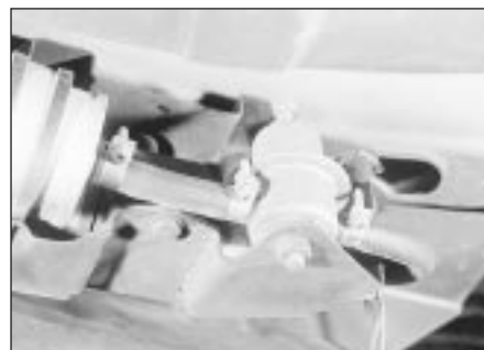
18.1 Fuel flow damper - models with semi-trailing arm rear axles
