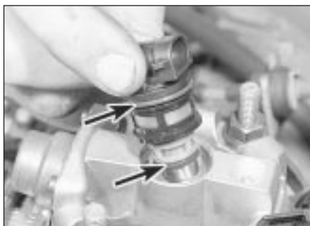
29.6 Renew injector sealing rings (arrowed)
