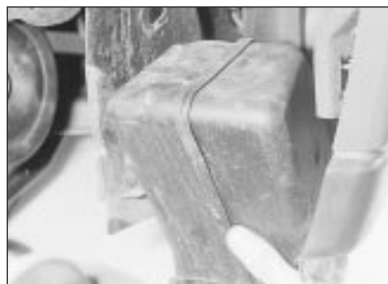
4.11B . . . and withdraw the resonance box
