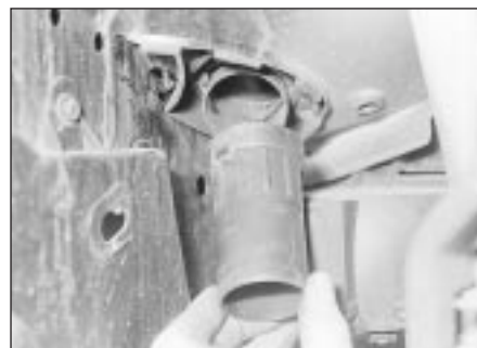
4.12 Removing the resonance box connector tube
