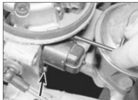
33.4A Unscrew retaining screws (second screw arrowed) . . .
