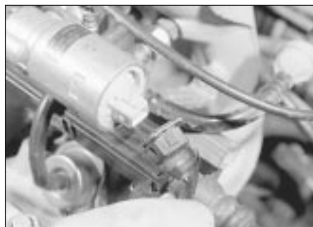
22.2 Disconnecting the idle speed adjuster wiring plug - SOHC models (except with Multec systems)
