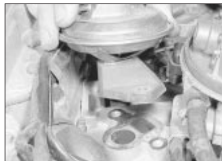
3.4B Withdrawing the exhaust gas recirculation valve
