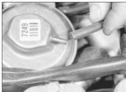
3.4 Disconnecting the vacuum hose from the exhaust gas recirculation valve
