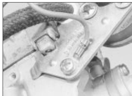
20.22 Secondary choke pull-down solenoid securing screw and earth lead
