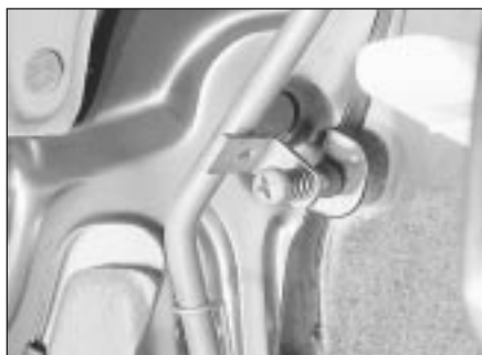
11.11 Throttle pedal stop screw
