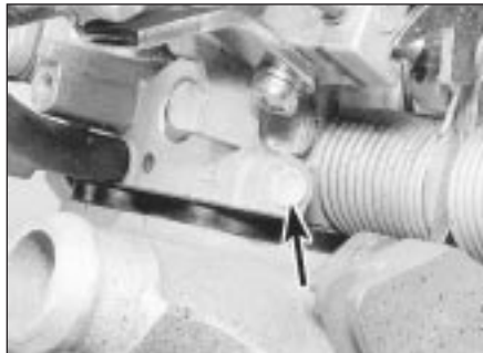
14.4 Tamperproof plug (arrowed) covering idle mixture adjustment screw
