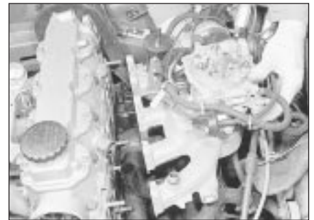
26.11 Withdrawing the inlet manifold - 1.6 litre model
