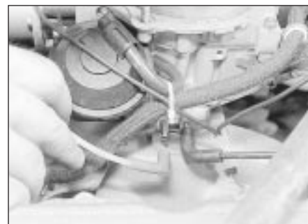
13.6 Disconnecting the air box vacuum pipe from the carburettor - 1.6 litre model
