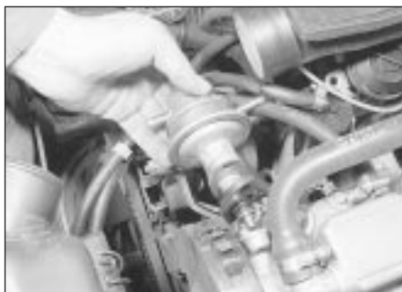
6.4 Withdrawing the fuel pump and plastic insulating block - 1.6 litre model
