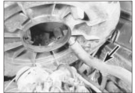
3.4 Disconnecting the crankcase ventilation hose (arrowed)
