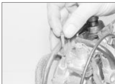
21.6 Refitting the carburettor fuel filter
