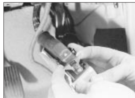
23.16 Releasing the Motronic module wiring plug clip - 2.0 litre model
