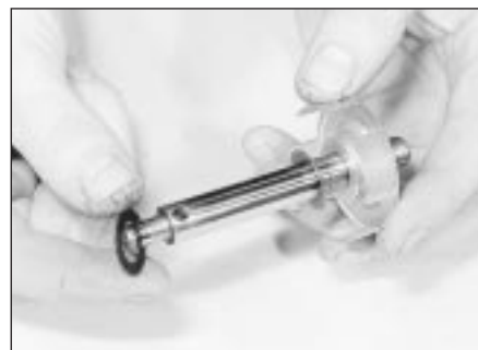
20.14 Recovering the thrustwashers from the shaft - 1.6 litre (Bosch distributor)
