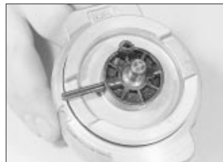
20.12 Removing the drive collar roll pin - 1.6 litre models (Bosch distributor)
