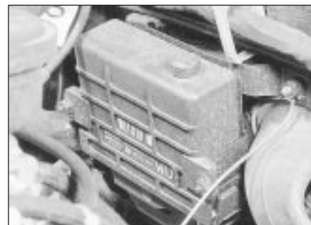
23.6 MSTS-i module location - 1.6 litre model
