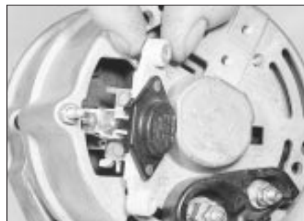
11.20B . . .and withdraw the brush holder/voltage regulator assembly - Bosch alternator
