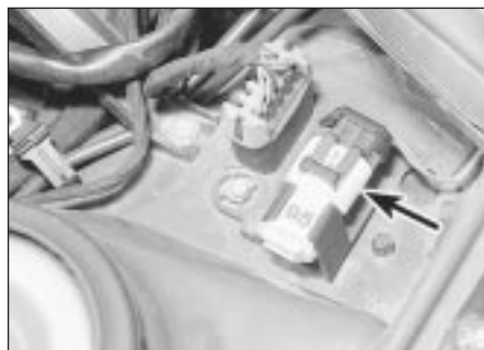
22.3 Octane coding plug (arrowed) - 2.0 litre model
