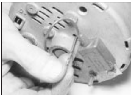
11.15 Withdrawing the twist drill used to retain the brushes - Delco-Remy alternator
