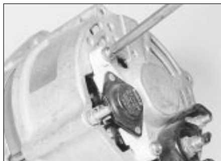
11.20A Remove the securing screws . . .
