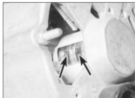
11.26 Alternator slip rings (arrowed) - Bosch alternator
