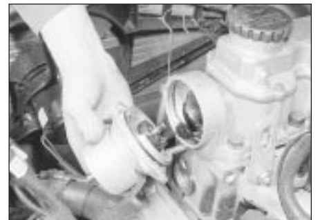
18.7C . . .and withdraw the distributor
