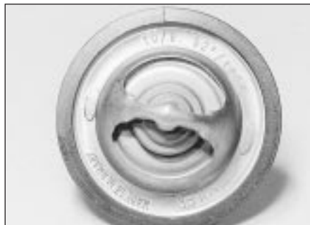
10.2 View of thermostat showing opening temperature markings - 1.6 litre model
