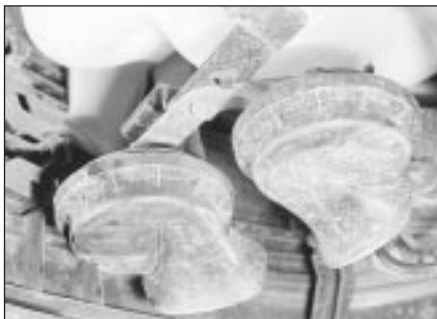
22.10 Horn mounting bracket securing bolt (arrowed) - twin horned model
