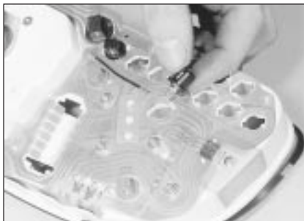
19.2 Withdrawing an instrument panel illumination lamp bulb
