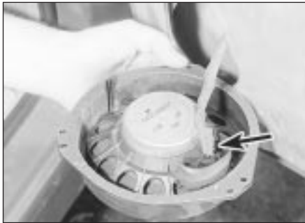
49.6 Withdrawing a front door-mounted speaker - wiring plug arrowed
