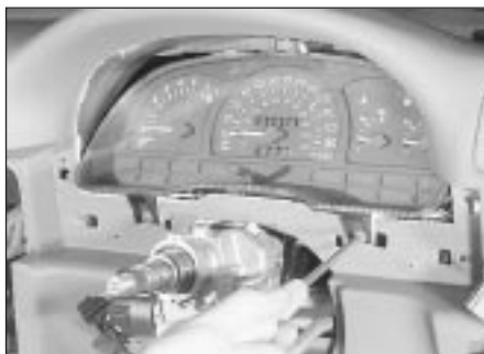
18.4 Unscrewing a lower instrument panel securing screw
