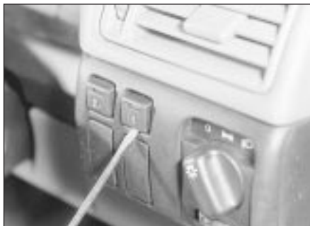
7.6 Prising a push-button switch from the facia
