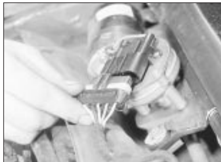
38.4 Disconnecting the windscreen wiper motor wiring plug
