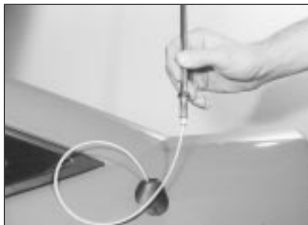
48.7 Push the mast assembly down, until it engages in the clutch mechanism
