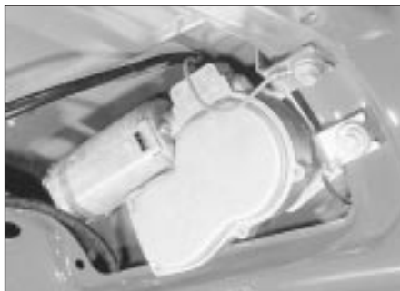
39.5 Tailgate wiper motor assembly. Note earth leads under heads of securing bolts
