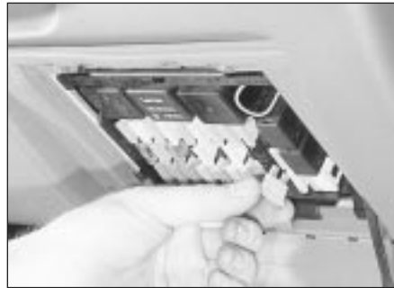
3.5 Removing a fuse - 2.0 litre model shown
