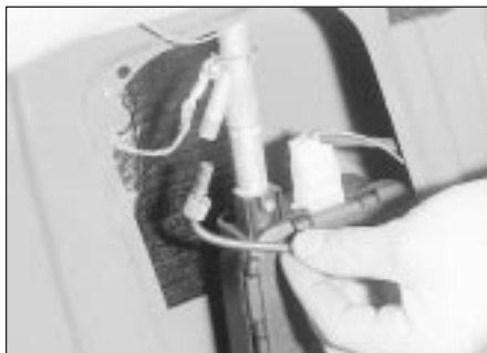
47.4B Disconnecting the aerial lead - electric aerial
