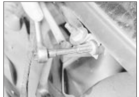
38.5A Unscrew the windscreen wiper motor/linkage assembly securing bolts . .
