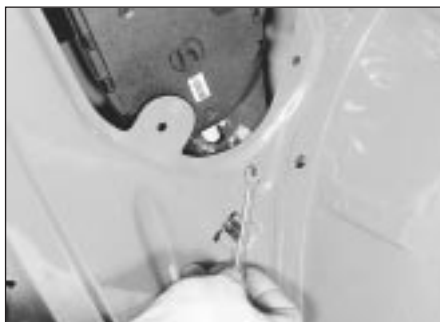
47.4A Unscrewing the radio aerial bracket securing screws - electric aerial
