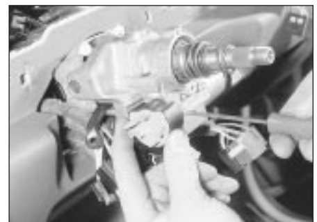
4.6 Removing an ignition switch securing screw
