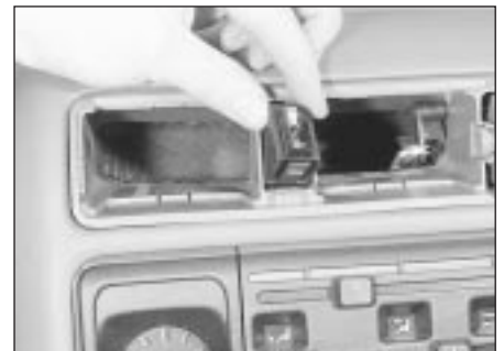
7.11 Withdrawing the hazard warning flasher switch from the facia
