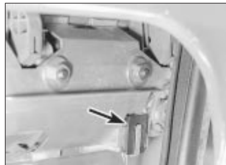
46.10 Central door locking operating microswitch (arrowed) in driver's door
