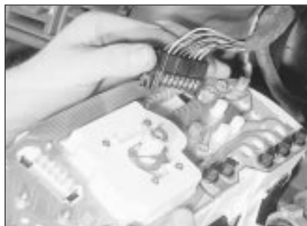
18.5 Disconnecting an instrument panel wiring plug. Note speedometer cable retaining clip (arrowed)
