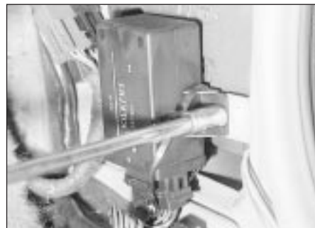
46.4 Unscrewing a central door locking control module securing nut
