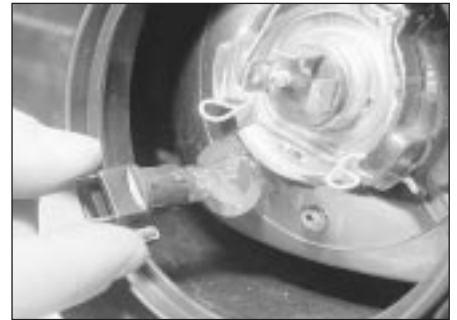
34.6 Pull the sidelamp bulbholder from the headlamp . . .
