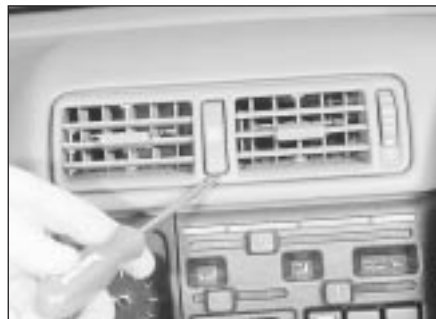
7.9 Prising the cap from the hazard warning flasher switch
