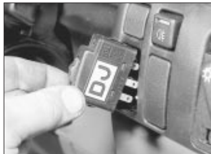
27.4 The headlamp aim adjustment switch - 1992-on models
