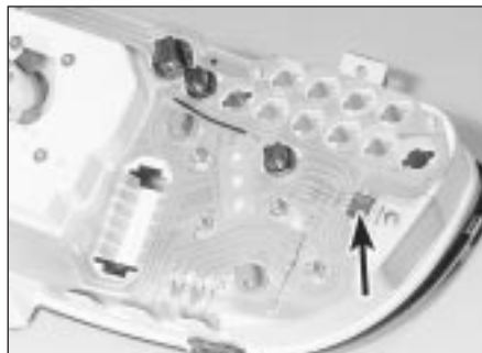
19.5 Instrument panel voltage stabiliser (arrowed)
