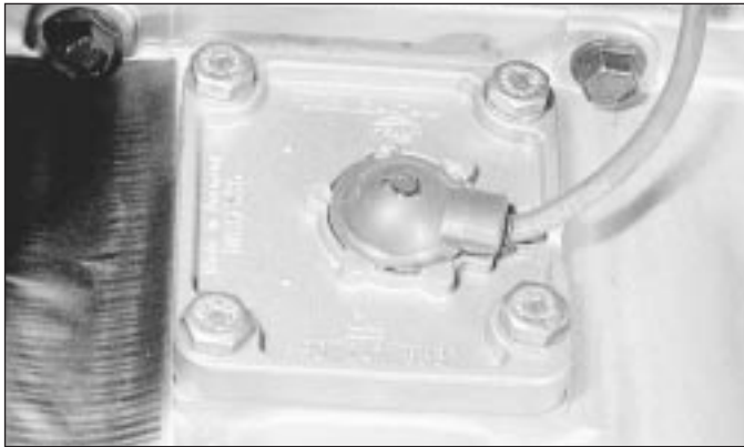
21.18 Engine oil level sensor - DOHC model
