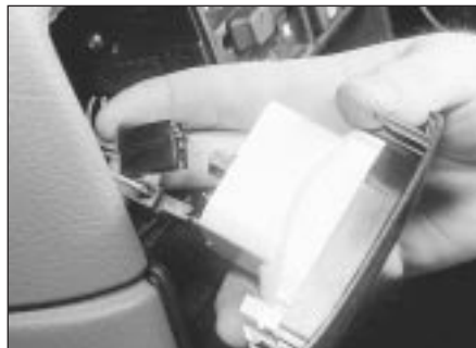
16.3 Disconnecting the wiring plugs from the clock
