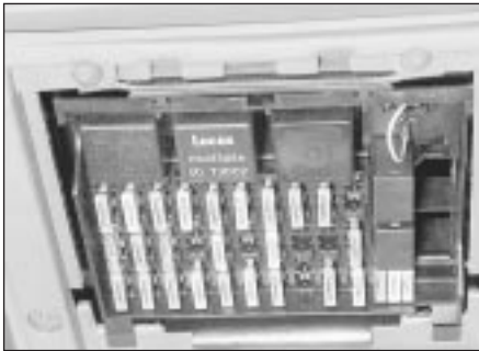
3.2 Main fuses and relays in fascia panel - 2.0 litre SRi model shown
