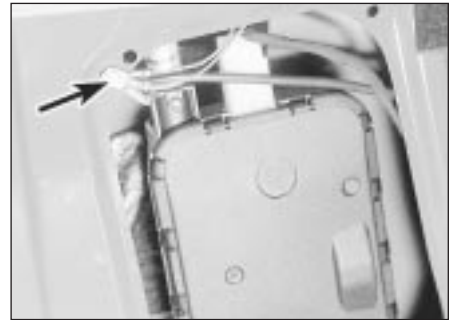
47.3 Radio aerial earth lead securing screw (arrowed) - electric aerial
