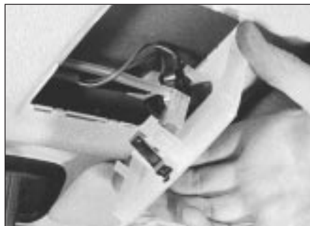
8.13a Interior light removal – 1.3 litre
