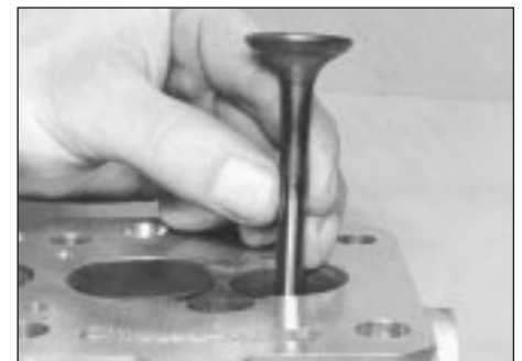
5.12 Removing a valve
