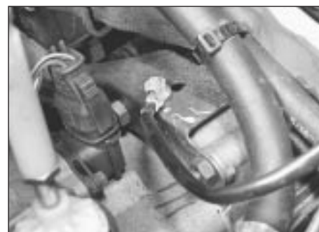
5.8c Earth strap to gearbox
