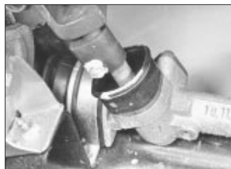
17.6 Steering gear pinion-to-lower column joint
