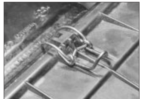
32.4a Unclip air cleaner cover . . .
