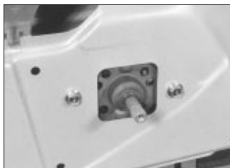
20.3a Window regulator securing bolts
