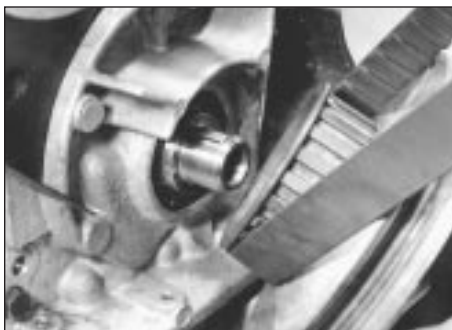
36.9 Fitting crankshaft sprocket and timing belt
