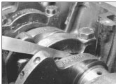
18.3 Checking crankshaft endfloat
