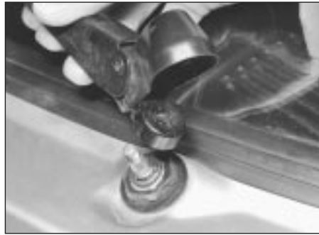
26.3 . . . and withdraw arm from spindle
