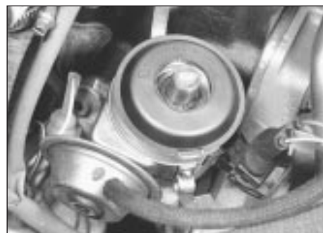
7.3b . . . and lift off the dust cap
