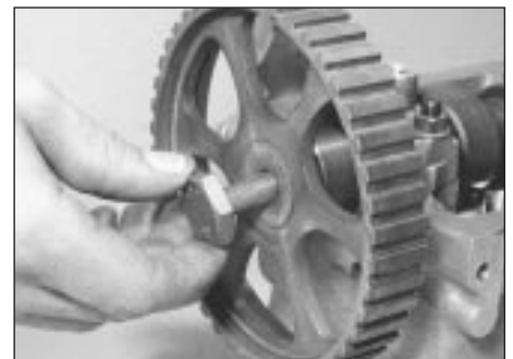
10.8 Fitting the camshaft sprocket bolt
