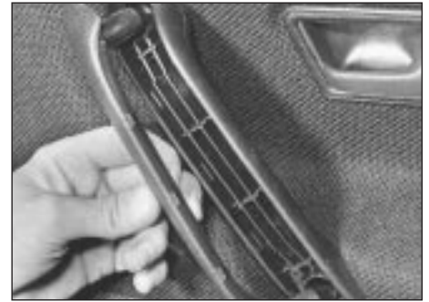
14.3a Removing door pull cover
