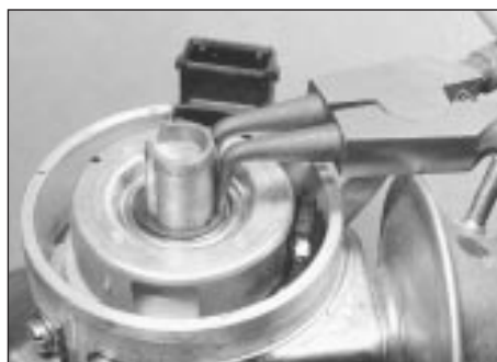
7.4a Remove the locking ring and rotor . . .
