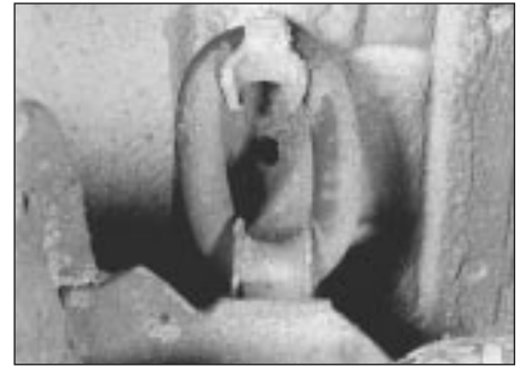
19.3 Check exhaust system mountings
