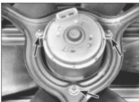
4.4 Cooling fan motor retaining nuts (arrowed)
