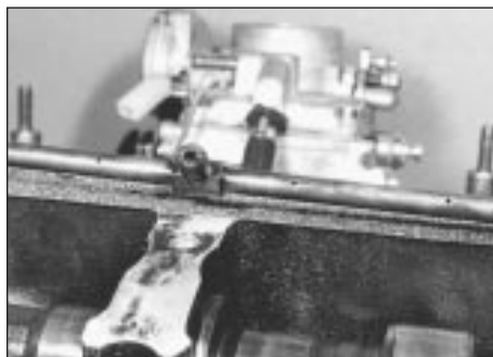
10.7 Removing oil spray tube
