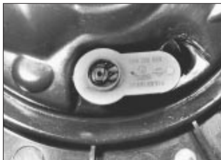
4.5 Upper view of air temperature sensor - 1.3 litre
