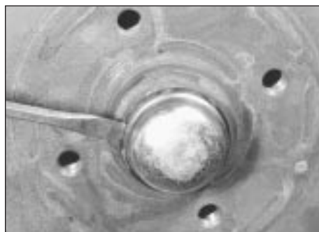
6.4a Remove the hub cap ...
