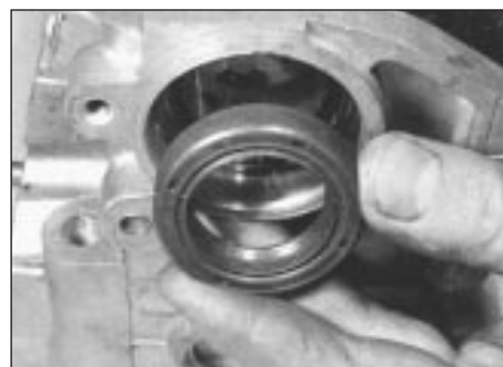
10.15 Removing camshaft oil seal
