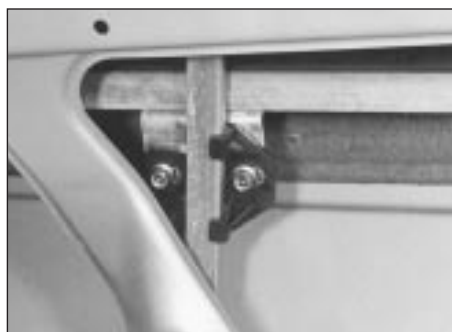
20.3b Lifting plate-to-window channel bolts
