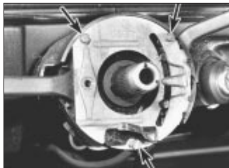
12.4 Combination switch retaining screws (arrowed)
