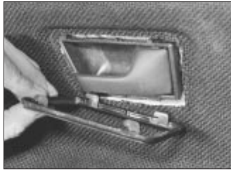
14.2 Removing door inner handle surround
