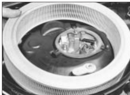
32.2 . . . and remove the element - 1.3 litre, carburettor
