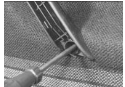
14.3b Removing door pull retaining screws
