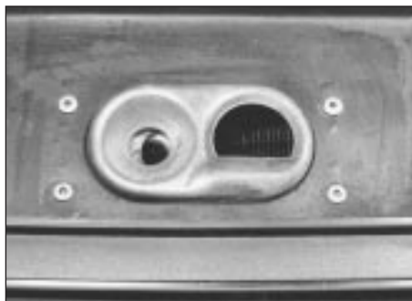
7.1 Bonnet lock and securing rivets
