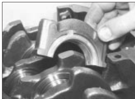
30.5 Fitting main bearing caps
