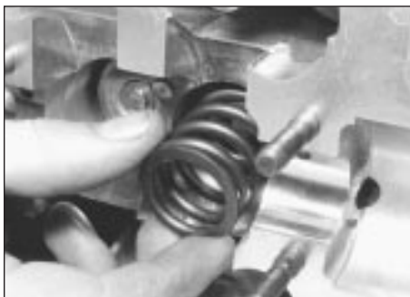
5.11a Removing an outer valve spring
