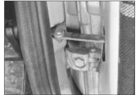
16.1 Door check strap and hinge
