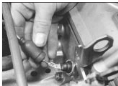
11.23c Oil pressure switch electrical connection
