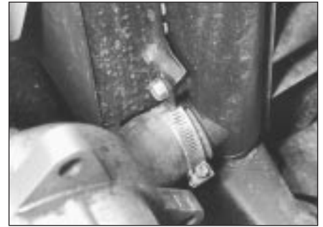
2.4b Radiator bottom hose connection - 1.8 litre
