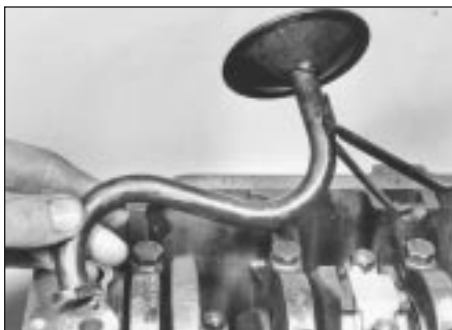
16.3 Removing oil pump pick-up tube and strainer
