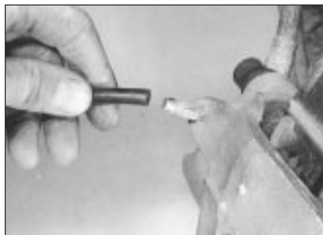
12.5 Connect bleed tube to bleed valve
