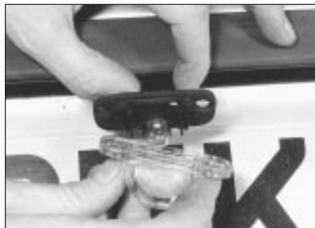
8.10 Number plate lens removal
