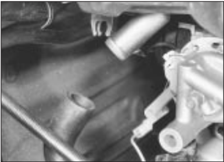
3.3b . . . and crankcase emission hose - 1.3 litre
