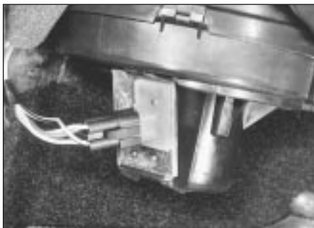
9.3 Blower unit and wiring connection
