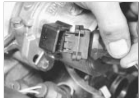
11.23a Ignition distributor electrical connection
