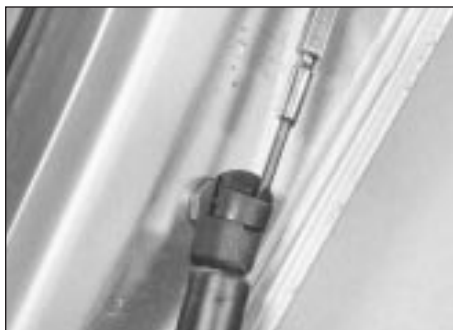
9.2a Releasing tailgate strut balljoint clip
