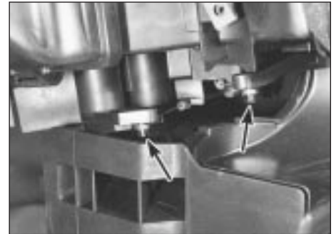
8.6c Control cable connections to flap valves at heater distribution box unit (arrowed)
