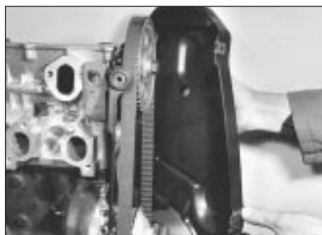
9.4 Removing timing cover
