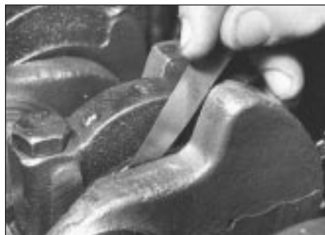
15.3 Checking crankshaft endfloat at No. 3 main bearing
