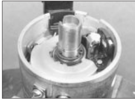
7.7 Hall sender unit, retaining ring and washers
