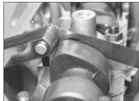
8.6 Measuring camshaft endfloat
