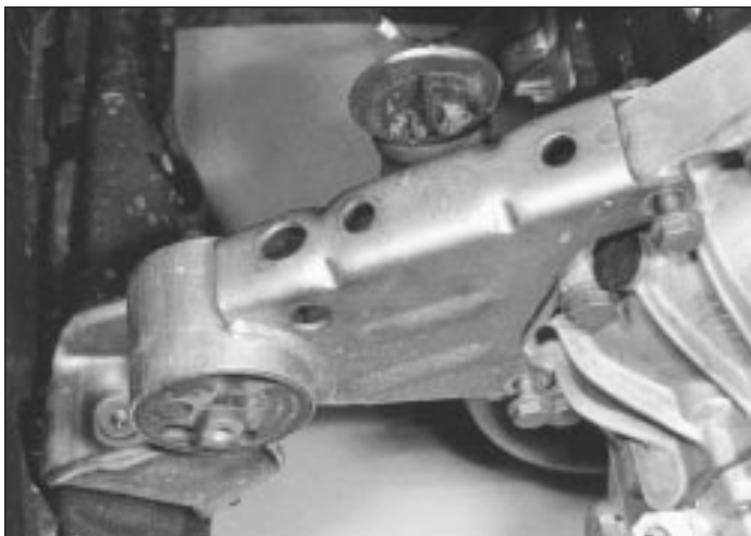
5.26b Unbolt and remove mounting unit
