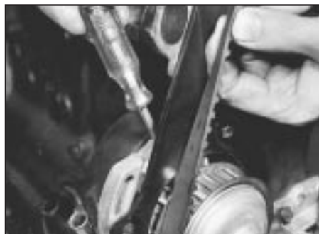
36.13 Tensioning timing belt
