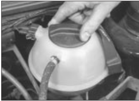
2.2 Removing expansion tank cap
