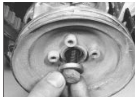
12.7 Removing crankshaft sprocket bolt and washer
