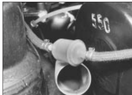
33.1 In-line fuel filter - 1.05 and 1.3 litre, carburettor
