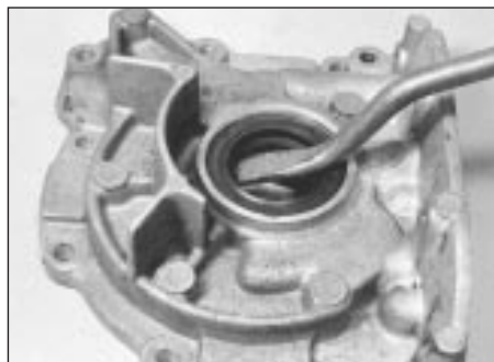
31.1 Prising out oil pump oil seal
