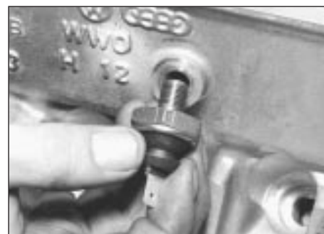
11.3 Refitting oil pressure switch
