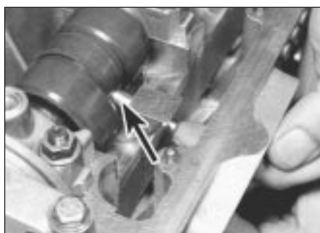
11.6 Fitting fuel pump plunger (arrowed)
