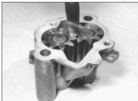
25.3 Checking oil pump gear backlash
