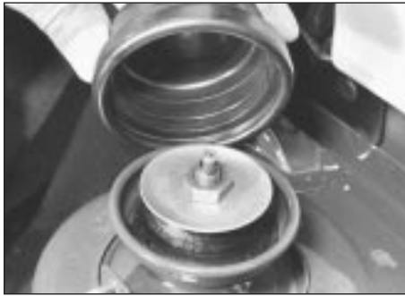
8.4 Removing rear suspension strut top cap
