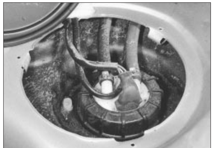
18.2 Fuel tank sender unit and connections
