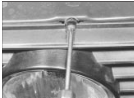
8.2 Undoing front grille retaining screws
