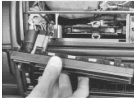
8.3b Unclip and withdraw trim panel
