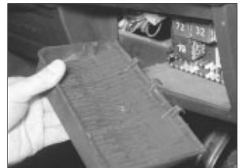
3.1 Removing fuse/relay unit cover
