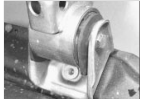
5.26a Undo front mounting through-bolt
