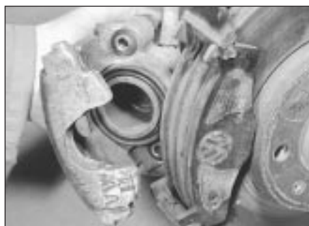
2.3b Removing the caliper
