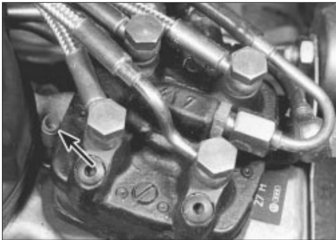
7.2 Idle CO adjustment screw location (arrowed)
