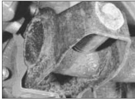
8.6 Rear suspension strut bottom mounting
