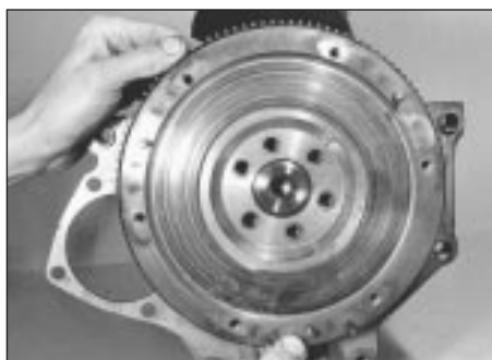
13.3 Removing flywheel
