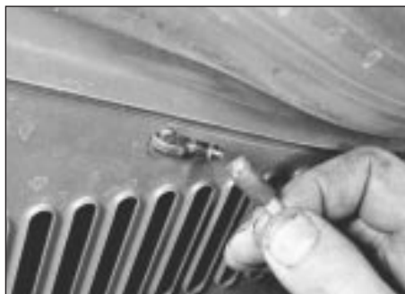
6.3 Disconnecting windscreen washer tubes from bonnet
