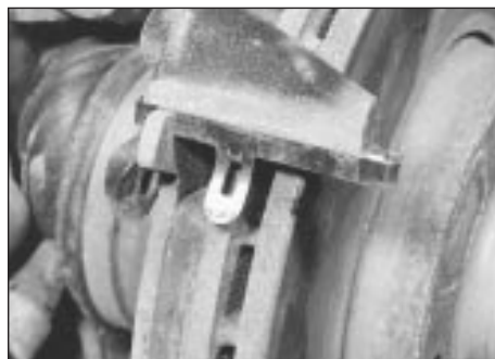
2.9 Pad retaining spring is located as shown
