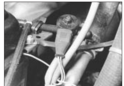
20.6 Fuel consumption gauge sender unit
