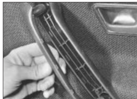
14.3a Removing door pull cover
