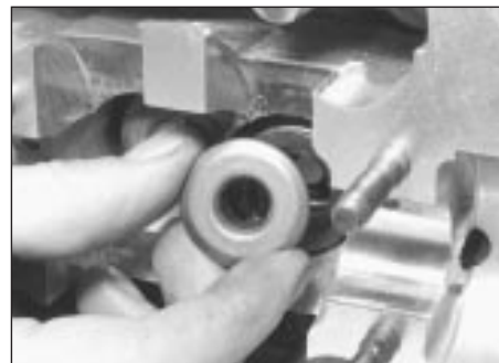
5.10 Removing valve spring upper seat
