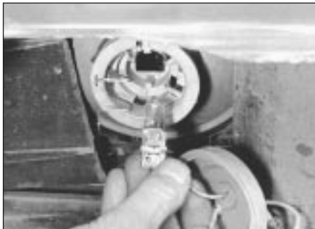
7.2 Bulb and holder removal from foglight
