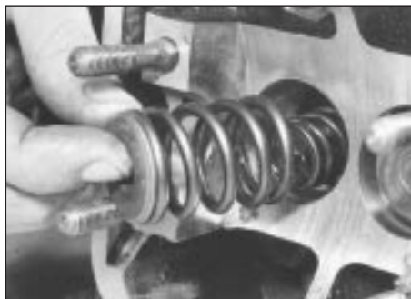
12.12b Locating valve springs and cap . . .
