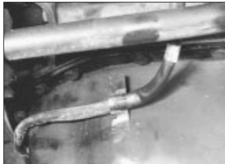
15.1 Alternator wire clip on sump
