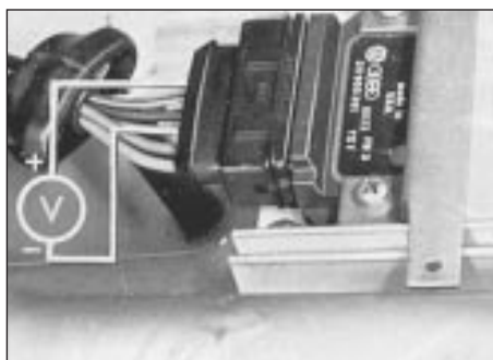
5.4 Voltmeter connection when testing Hall sender
