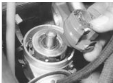
7.3a Pull free the rotor . . .
