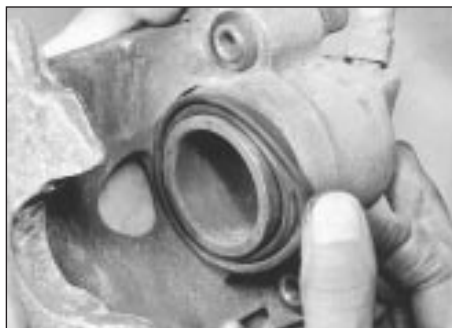
3.5 Removing the dust seal
