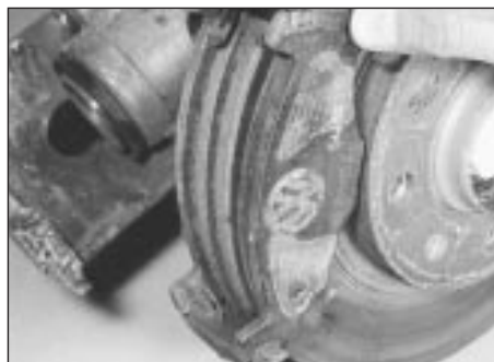
2.10 Refitting front brake pads
