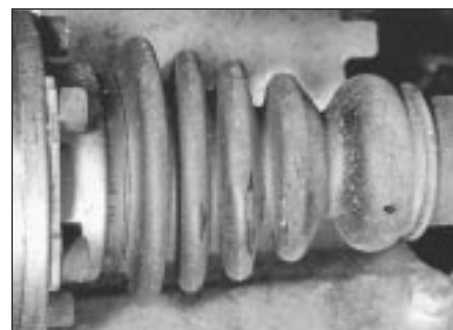
24.2 Inspect condition of each CV joint boot
