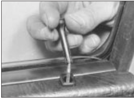
14.1 Unscrewing door locking knob
