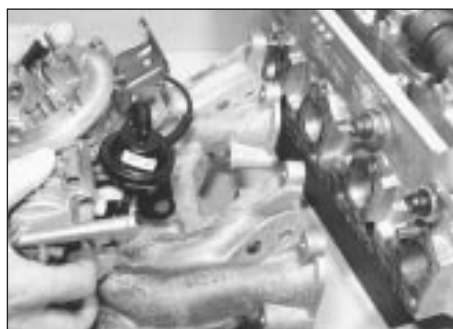
11.2b Fitting inlet manifold complete with carburettor
