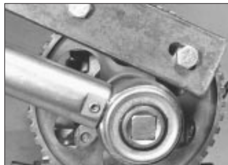
35.5 Method of tightening camshaft sprocket bolt
