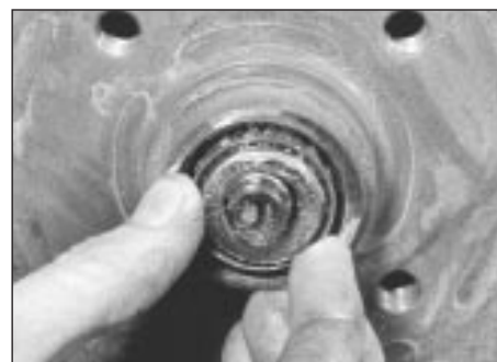
6.5c ... and outer bearing
