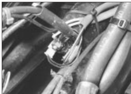
10.4 Starting motor solenoid wiring connections – 1.3 litre
