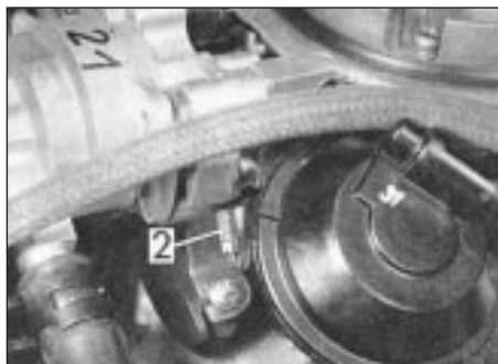
16.10 Fast idle speed adjustment screw (2)
