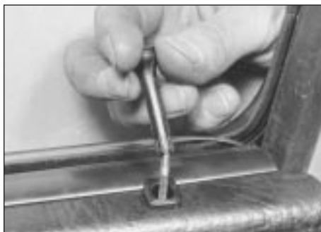
14.1 Unscrewing door locking knob
