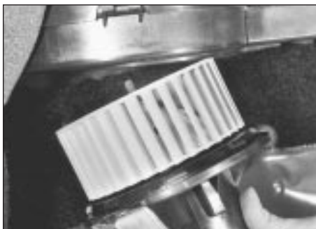
9.4 Blower unit withdrawal from housing
