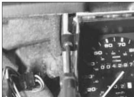
16.3 Instrument panel screw removal
