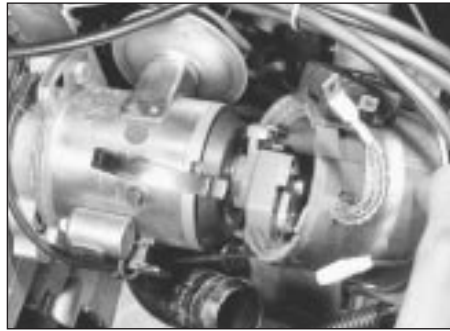
11.2 Withdraw distributor cap and screen ring
