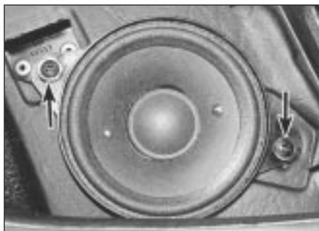
32.3 Facia-mounted loudspeaker retaining screws (arrowed)
