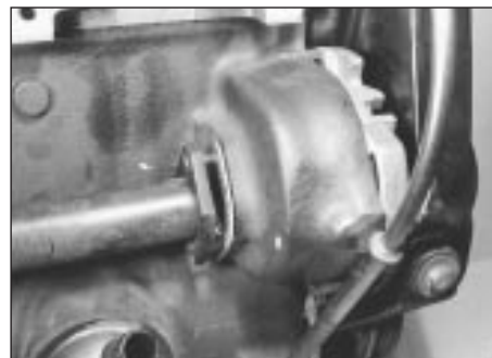
8.1d Removing engine rear coolant pipe
