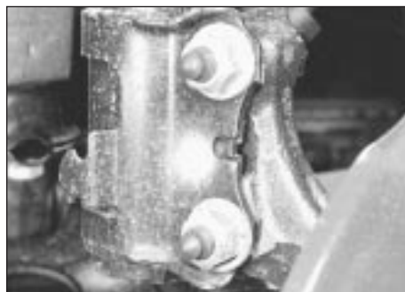
2.7 Strut-to-front wheel bearing housing retaining nuts/bolts
