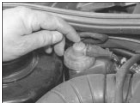
5.4 Check brake fluid level warning device
