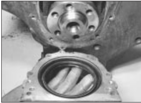
14.13a Withdrawing crankshaft rear oil seal housing . . .
