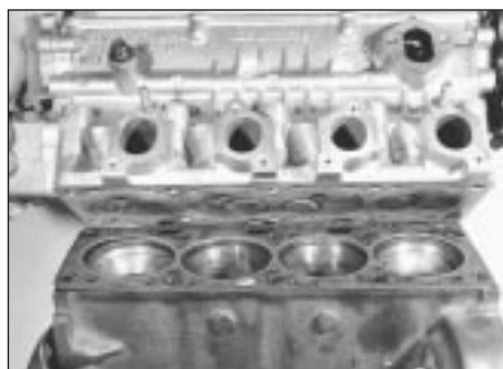
9.9 Removing cylinder head . . .
