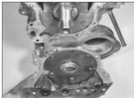
16.4a Removing oil pump . . .
