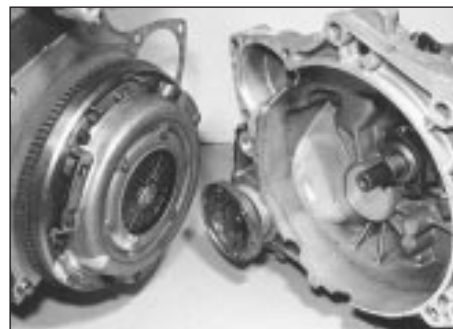
6.6b . . . then separate engine and transmission
