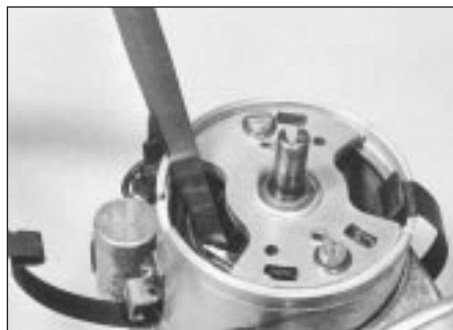
16.10a Checking contact breaker points gap
