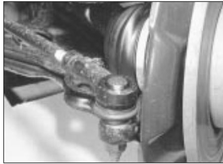
15.1 Right-hand adjustable balljoint
