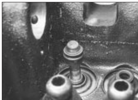
34.4 . . . then fit the new oil seal
