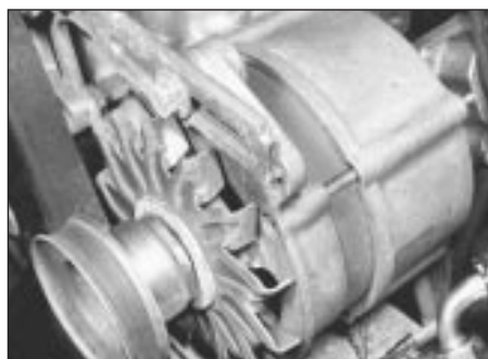
13.4b Alternator drivebelt tensioner link - 1.8 litre
