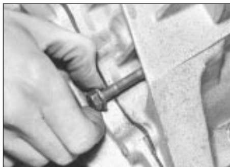
6.6a Undo securing bolts (recessed bolt shown) . . .
