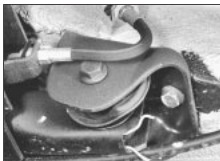
9.7 Axle beam pivot bolt head fitting position
