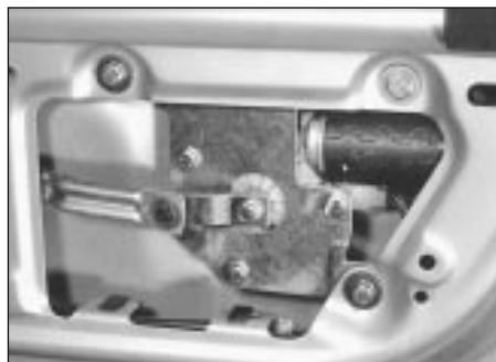
28.4b Rear wiper motor mounting in tailgate
