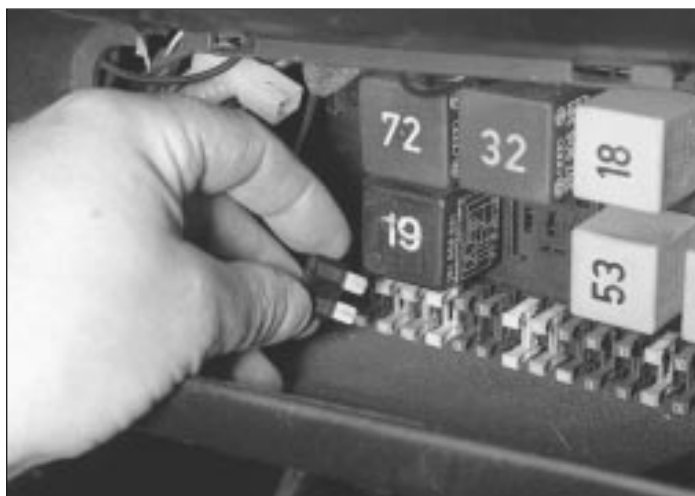
3.2 Removing a fuse
