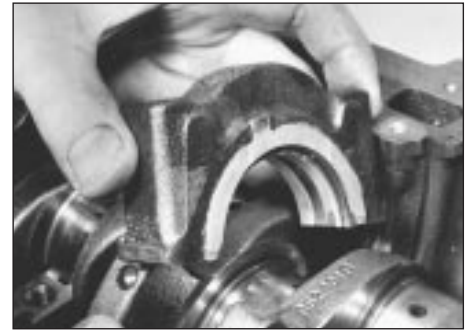
29.4 Fitting centre main bearing cap
