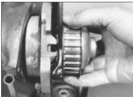
6.6 Withdrawing coolant pump
