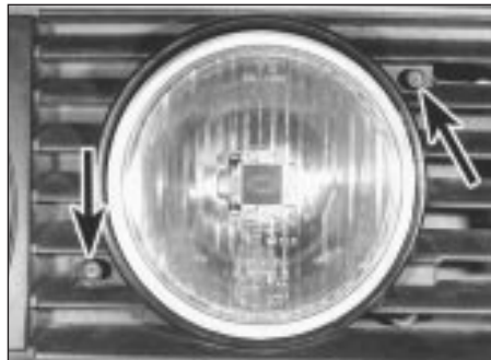
7.4 Foglight beam alignment adjuster screws (arrowed)
