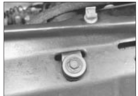
3.5 Radiator central retaining bolt and bracket
