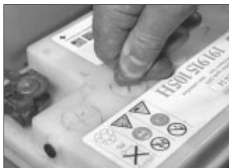
7.3a Remove battery filler caps . . .
