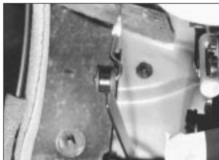
10.5 Accelerator cable-to-pedal attachment
