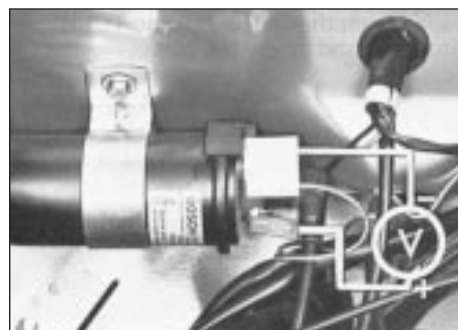
4.6b Voltmeter connection to coil when testing ignition switch unit and coil
