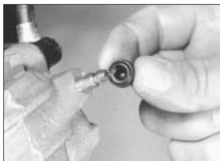
12.23 Fit bleed valve the protector cap
