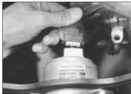
3.3b Detach cooling fan lead connector
