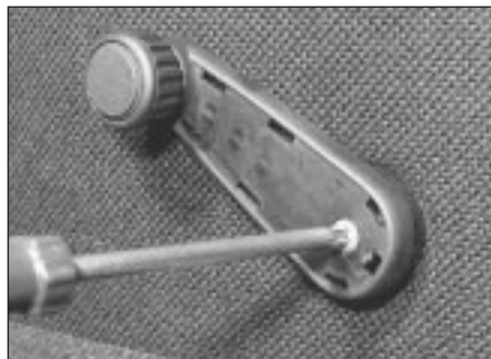
14.4b . . . and handle retaining screw
