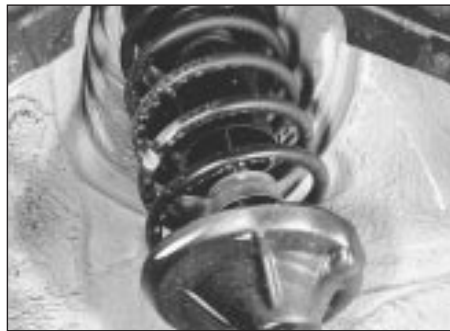
29.4 Check shock absorbers for leakage
