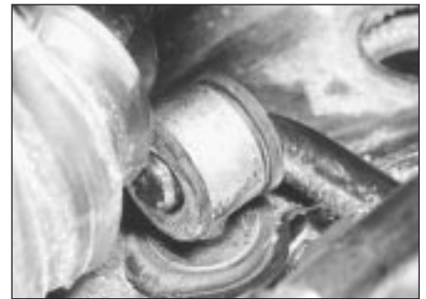
4.5 Anti-roll bar location in eye bolt
