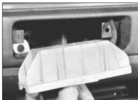
8.6 Front indicator lamp unit removal
