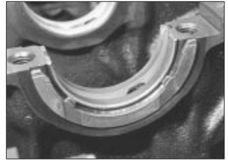
30.3c . . . together with thrustwashers
