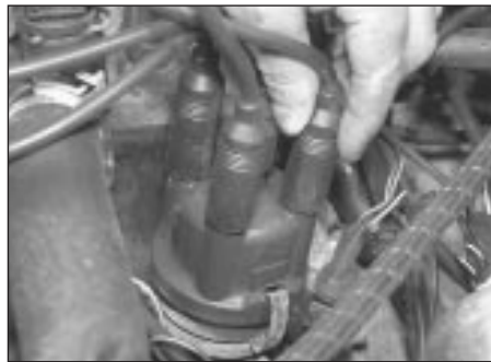
6.5 Ensure all HT lead connections are secure
