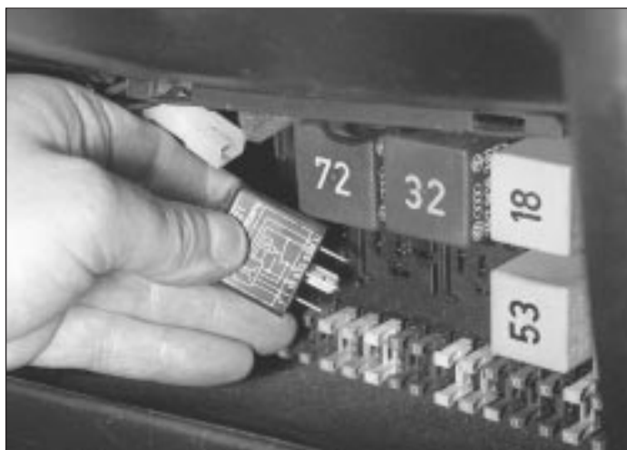
3.3 Removing a relay
