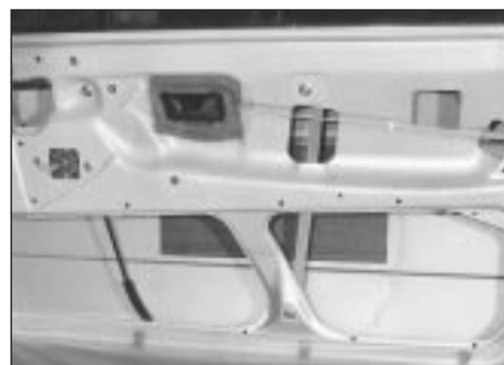
14.10 Plastic cover peeled back for access to door components
