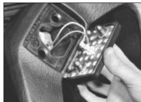
11.3a Removing steering wheel centre cover - 1.3 litre
