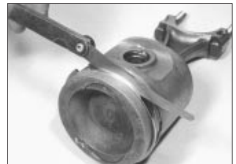
23.7b Checking piston ring-to-groove wall clearance
