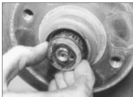
4.15 ... followed by the outer washer and bearing
