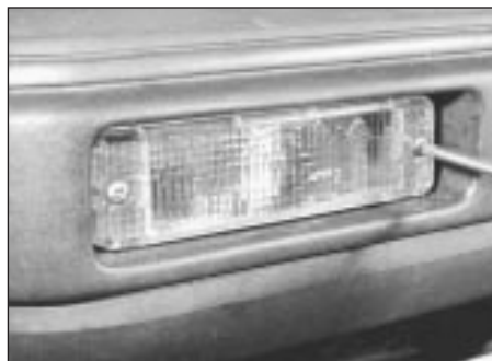
8.4 Front indicator lens removal
