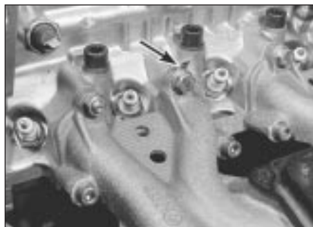
19.6 Inlet manifold-to-cylinder head securing nuts and bolts
