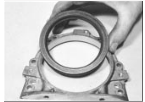
14.14 Remove crankshaft rear oil seal from housing
