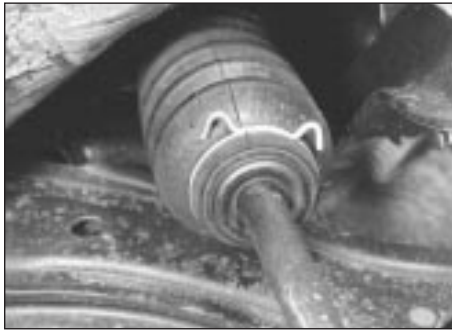
15.4 Steering tie-rod bellows and retaining clip
