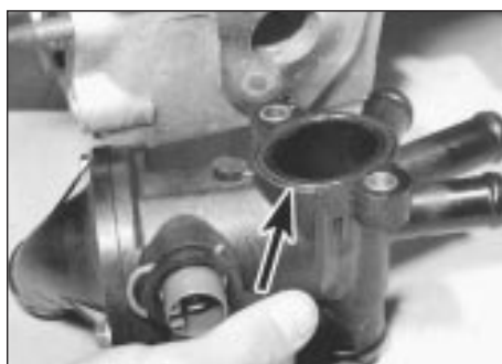
11.4 O-ring (arrowed) in thermostat housing
