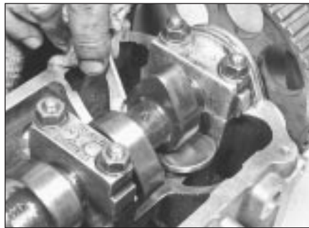
12.12 Removing a tappet bucket shim - 1.6 and 1.8 litre
