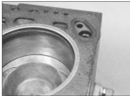
36.2 Correct fitting of cylinder head gasket
