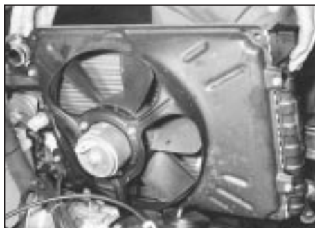
3.8 Lifting out radiator and cooling fan assembly
