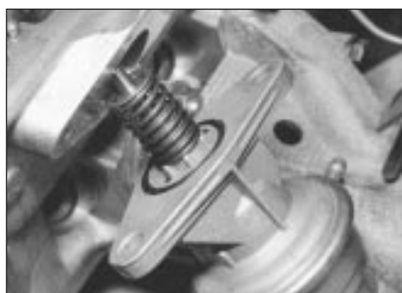
11.7a Fitting fuel pump
