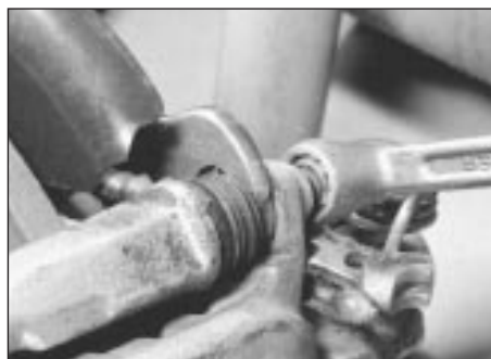
2.16 Rear caliper bolt removal Prevent guide pin from turning with open-ended spanner
