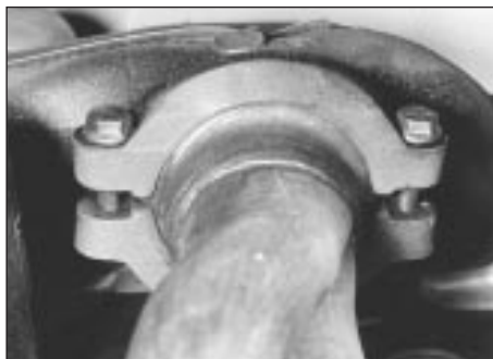
19.10 Exhaust downpipe-to-manifold flange connection - 1.3 litre
