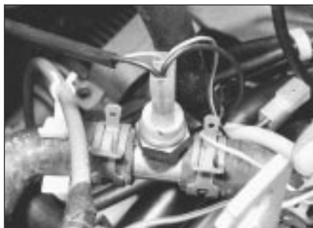
7.11 Temperature sender unit thermo-switch location - 1.05 and 1.3 litre
