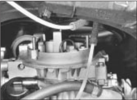
3.3a Disconnecting temperature sensor hose . . .
