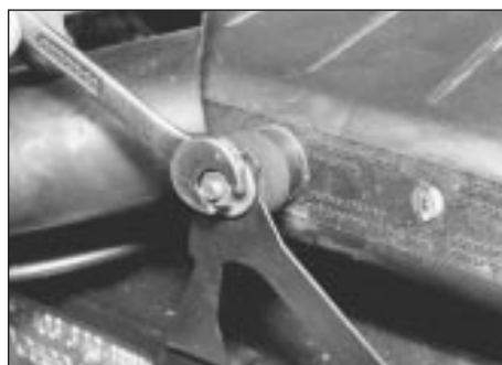
32.4b . . . loosen front mounting nut . . .
