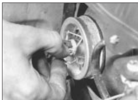
4.3 Squeeze bulb retaining clips . . .
