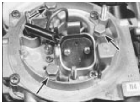
13.8 Carburettor securing bolts (arrowed) – Pierburg/Solex 2E3
