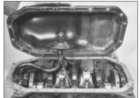
15.2 Removing the sump
