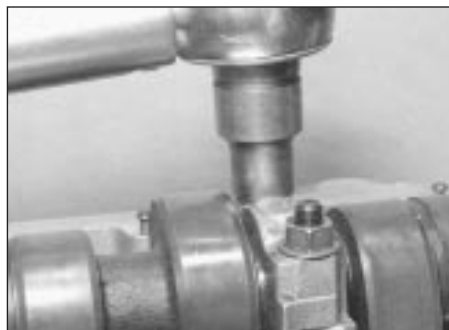
10.5 Tightening a camshaft bearing cap nut
