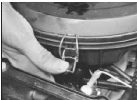
32.1 Unclip the air cleaner lid . . .
