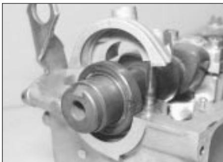
10.3 Camshaft oil seal
