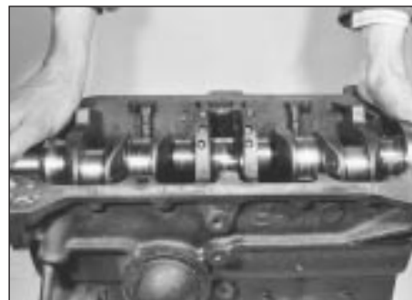
18.6 Removing crankshaft
