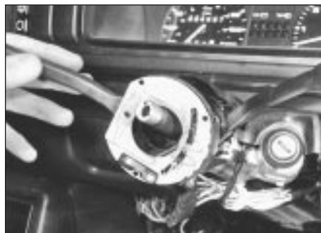
12.6 Removing indicator switch . . .
