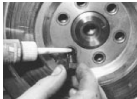
33.3 Applying liquid locking fluid to flywheel bolts
