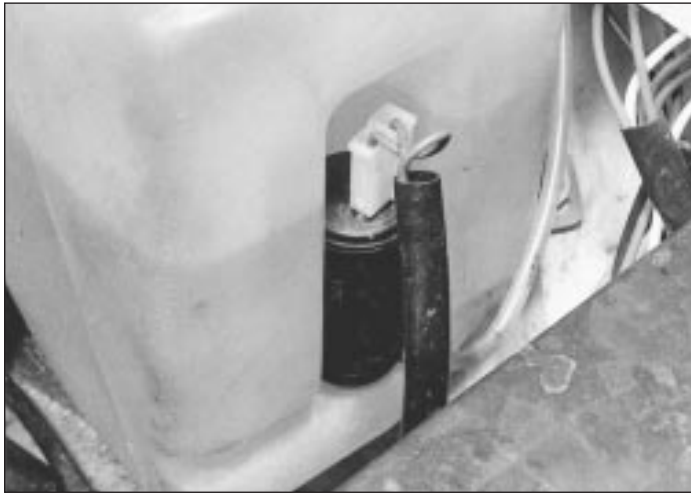
30.1 Windscreen washer pump and wire connector
