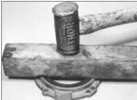
14.16 Installing new crankshaft rear oil seal
