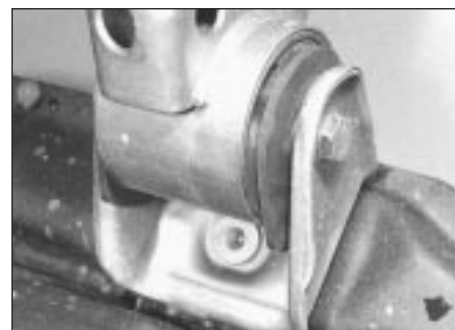
5.25a Engine/gearbox unit front mounting
