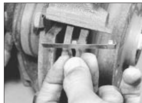
2.5 Removing a pad retaining spring
