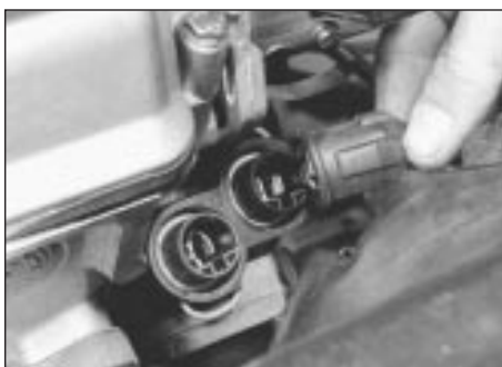
11.23b Coolant temperature switch/sender electrical connection
