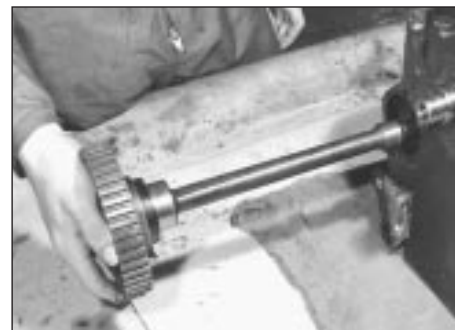
16.5b Withdrawing intermediate shaft
