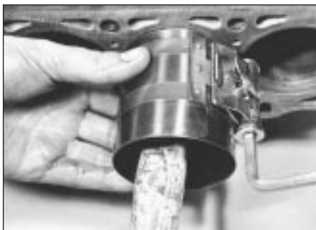
30.4 Using a piston ring compressor
