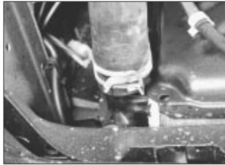
2.4a Radiator bottom hose connection - 1.3 litre
