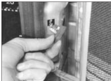
14.3 Door courtesy light switch removal
