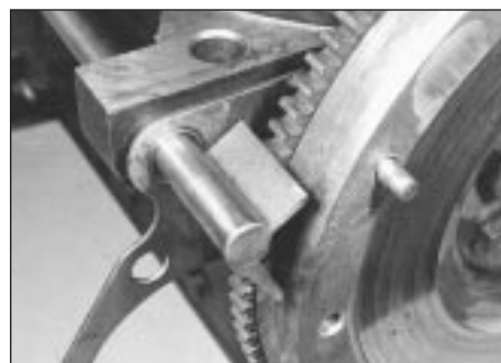
13.2 One method of holding the flywheel stationary
