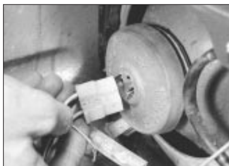
4.1 Detaching headlamp bulb connector
