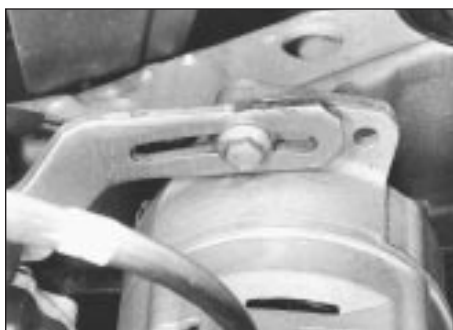
13.4a Alternator drivebelt tensioner link - 1.3 litre
