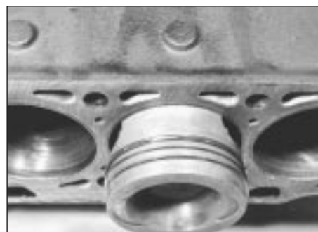
17.8 Removing a piston
