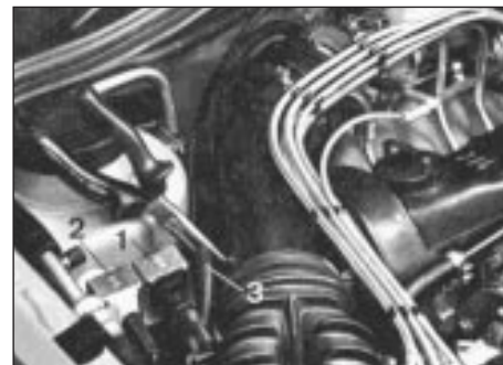
6.1 Idle speed boost valve check
