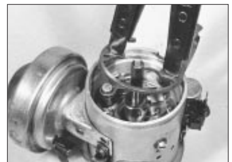
7.10b Removing bearing plate retaining ring
