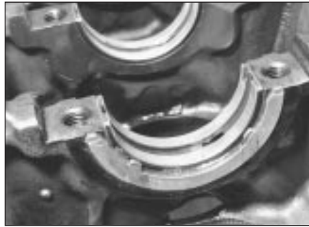
29.3 Thrustwasher location on centre main bearing
