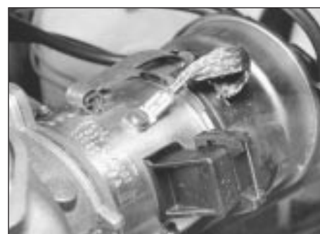
11.10 Fitting distributor cap and earth lead
