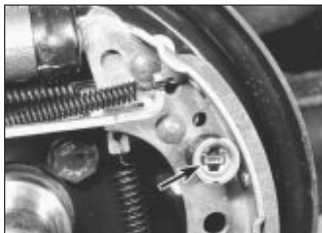
6.8 Brake shoe steady spring and cup (arrowed)
