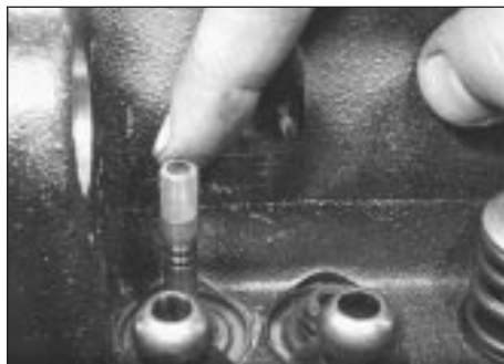
34.3 Locate plastic sleeve on valve stem . . .
