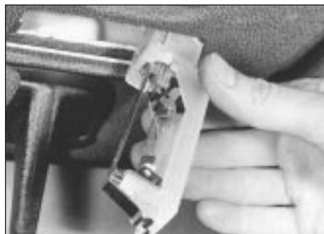
8.13b Interior light removal – 1.8 litre
