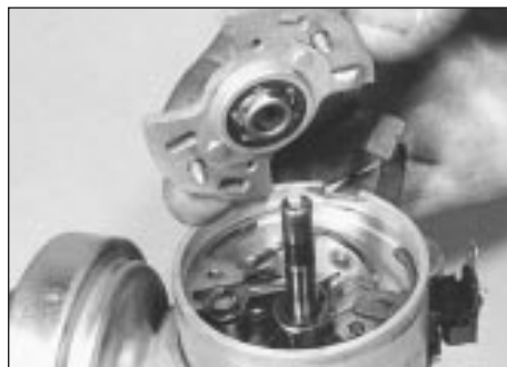
16.3 Removing the bearing plate - 1.05 and 1.3 litre
