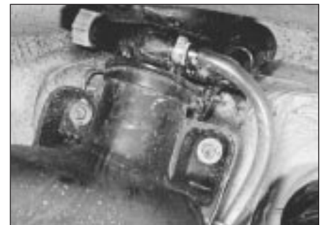
7.6 Fuel filler breather valve and hose
