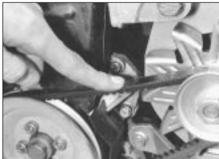
13.2 Checking alternator drivebelt tension
