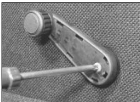
14.4b . . . and handle retaining screw
