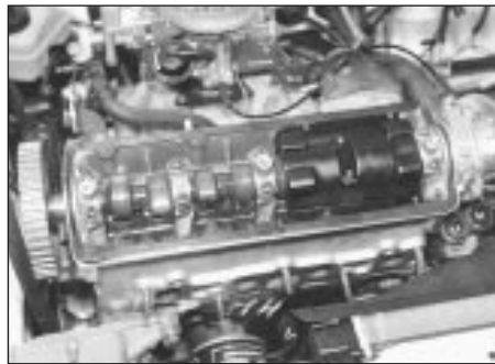
11.17 Plastic oil shield correctly located
