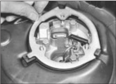
3.2 Removing air cleaner body retaining ring - 1.3 litre
