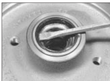
8.3 Prising out brake drum oil seal
