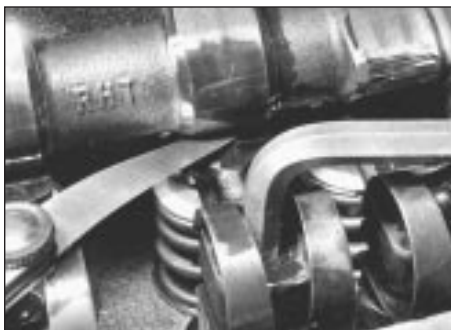
12.4 Adjusting a valve clearance - 1.05 and 1.3 litre
