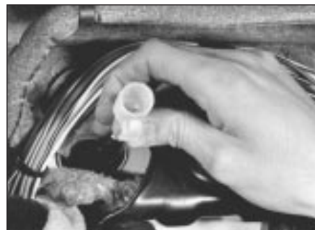
16.4 Disconnect speedometer cable
