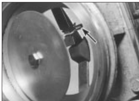
14.6 Airflow sensor plate adjustment clip (arrowed)
