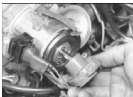
11.9 Fitting rotor arm
