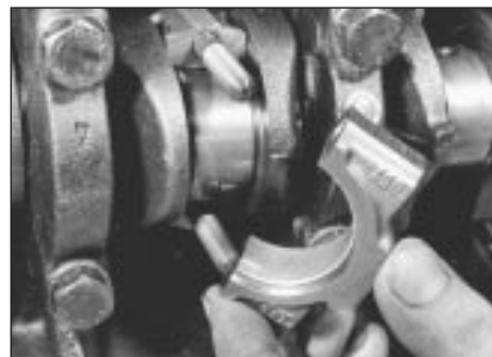
17.7 Withdrawing a big-end cap
