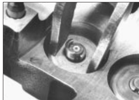
12.12c . . . and valve collets
