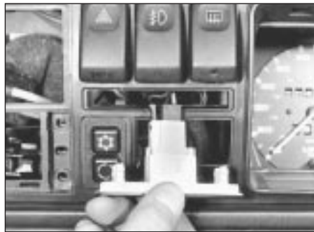
10.2 Warning lamp cluster removal
