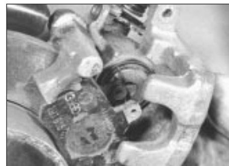
2.17 Rear brake caliper removal
