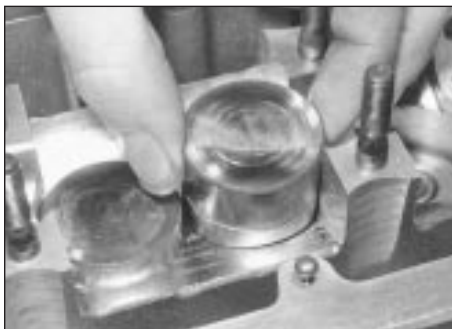
5.4 Removing an hydraulic bucket tappet
