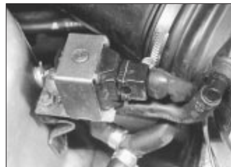
5.2 Increased idling speed valve (air conditioned models)
