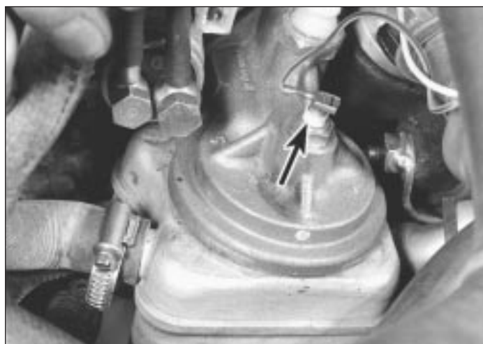
5.39 Oil temperature sender (arrowed)
