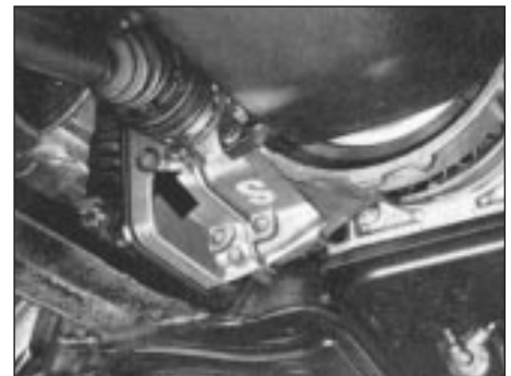
35.10 Final drive unit oil filler/level plug (arrowed)
