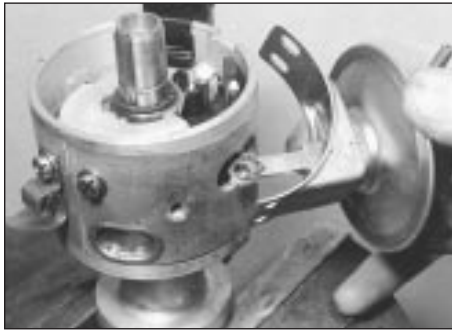
7.5 Vacuum unit removal
