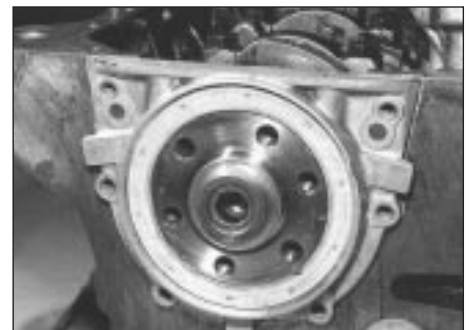
30.9 Fitting crankshaft rear oil seal and flange
