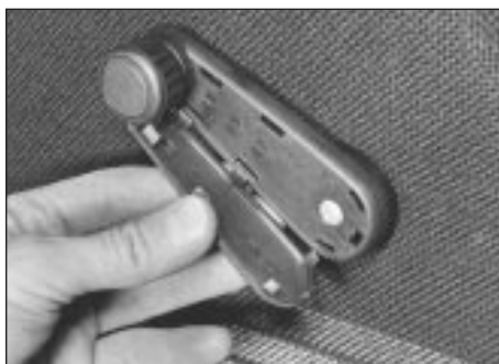
14.4a Remove window regulator handle cover . . .
