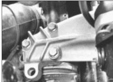
5.24 Engine mounting/bearer - right-hand
