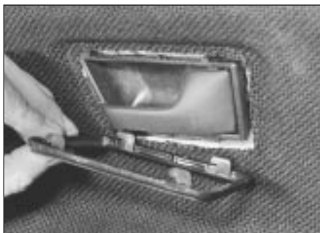
14.2 Removing door inner handle surround
