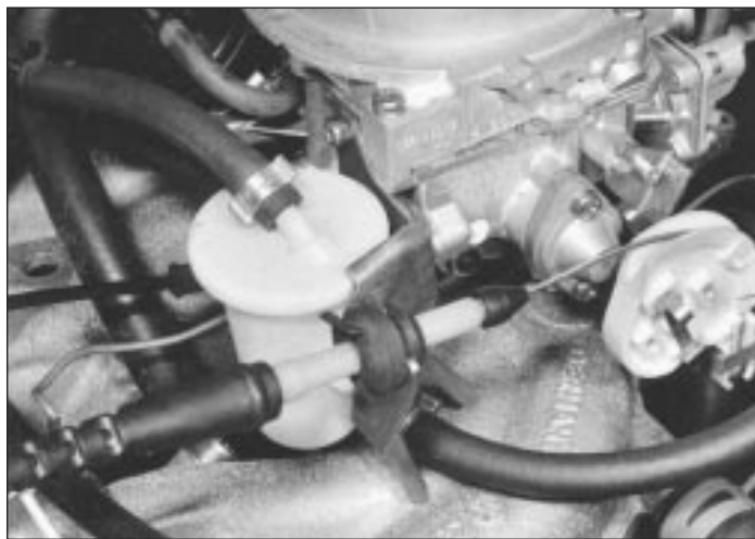
10.3 Accelerator cable to carburettor throttle control
