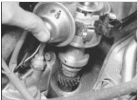
6.6a Distributor removal - 1.8 litre engine
