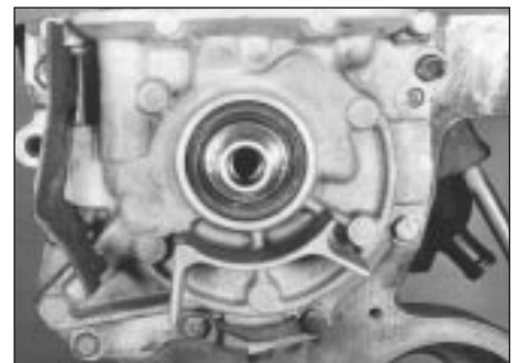
31.4 Fitted location of oil pump
