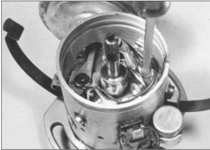
16.10b Adjusting contact breaker points gap
