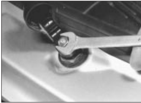
26.2 Undo wiper arm nut . . .
