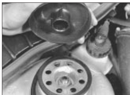
2.3 Removing front suspension strut top cap
