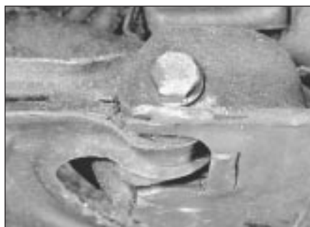
7.4 Track control arm pivot bolt
