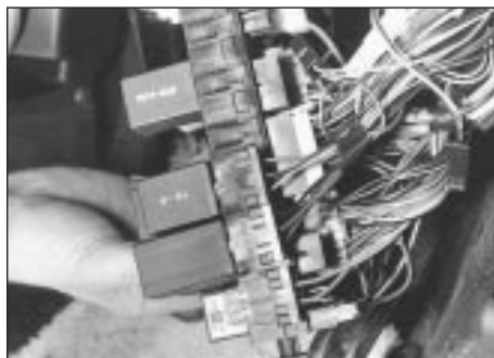
3.5 Fuse/relay unit removal, showing rear connections
