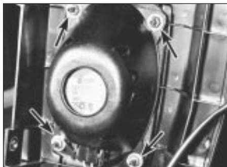
32.5 Luggage compartment loudspeaker retaining nuts (arrowed)
