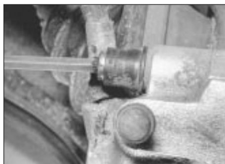
2.3a Caliper securing bolt removal
