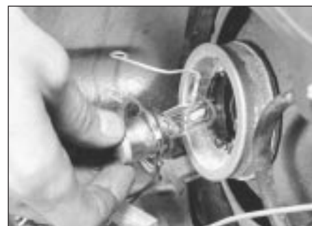
4.4 . . . and withdraw headlamp bulb
