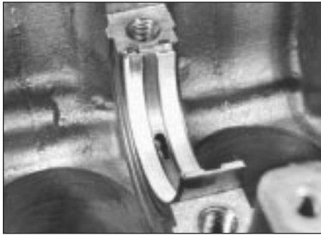
29.2 Fitting centre main bearing shell
