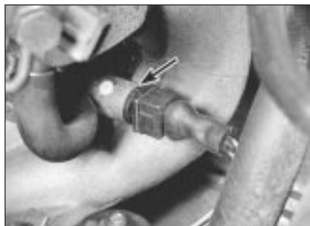
10.3 Auxiliary air valve (arrowed)
