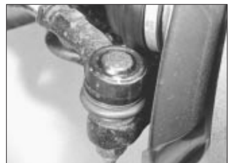
28.2 Inspect balljoint dust covers
