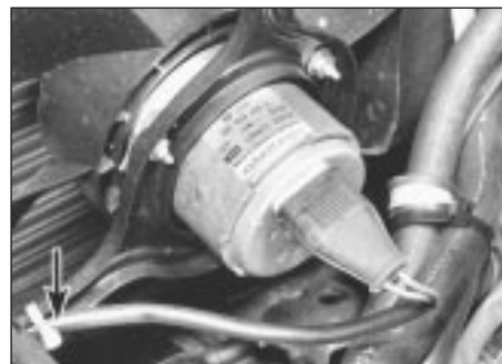
3.15 Secure fan lead with plastic clip (arrowed)
