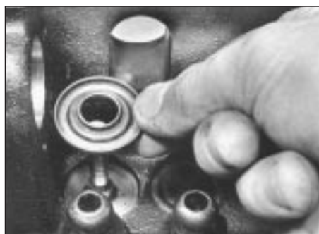
11.4 . . . and valve spring lower seats
