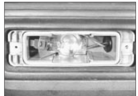
8.5 Front indicator lamp bulb
