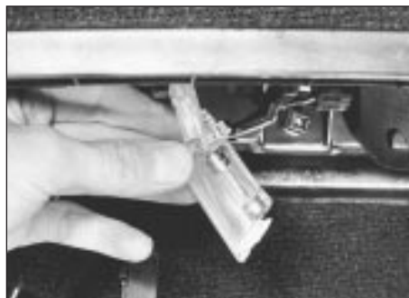
8.16 Luggage compartment lamp lens removal
