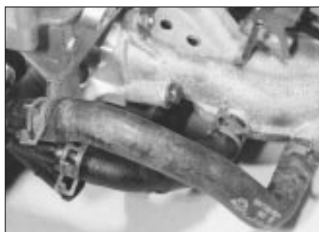
11.5 Coolant hoses in position
