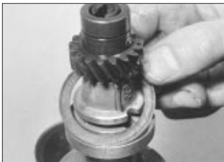
6.6b The gasket must be removed
