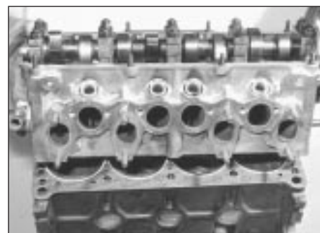
34.3a Lowering cylinder head onto block
