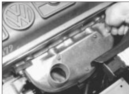
11.20 Fitting hot air shroud
