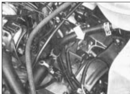
22.4 Gearbox filler/level plug location (arrowed) - 084 gearbox
