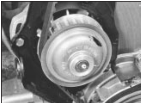
6.5 Disengage timing belt from coolant pump sprocket
