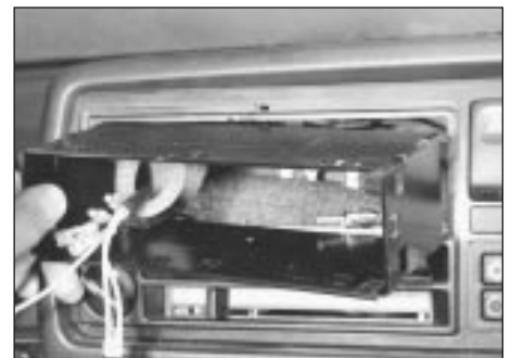
31.6 Radio/cassette container removal
