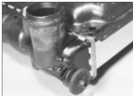
3.13 Radiator lower mounting rubber
