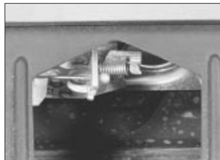
7.4 Bonnet release cable-to-lock attachment
