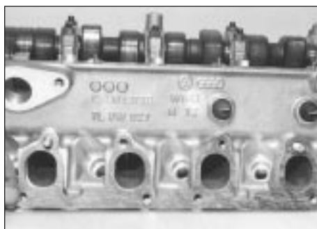
11.2a Fitting a new inlet manifold gasket
