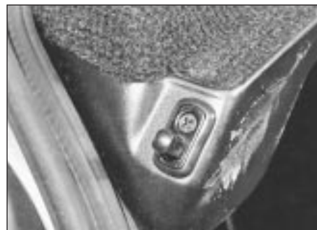
14.2 Tailgate actuated luggage compartment light switch
