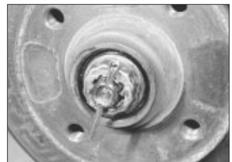
4.14 ... remove the split pin and lock ring ...
