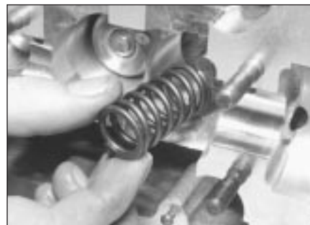
5.11b Removing an inner valve spring
