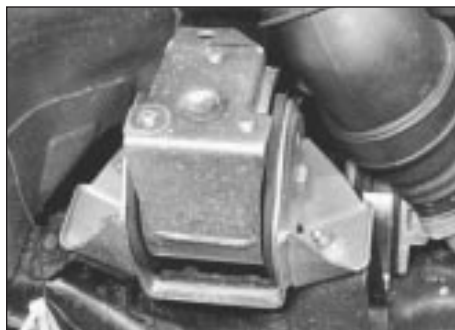
8.1b Right-hand rear mounting viewed from above
