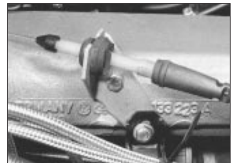
8.10 Accelerator cable adjuster and support bracket
