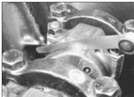
17.4 Checking connecting rod endfloat
