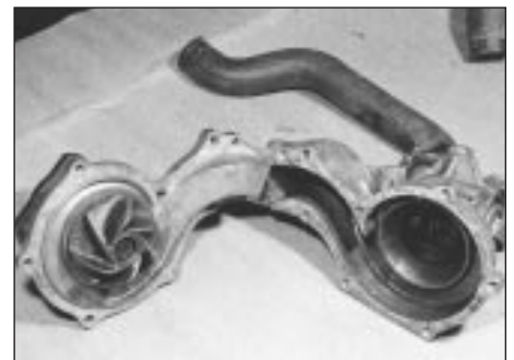
6.17 Two halves of coolant pump - 1.6 and 1.8 litre
