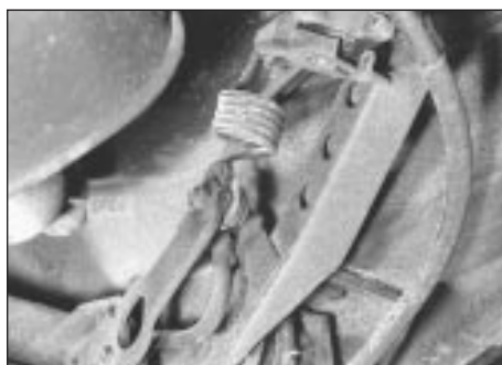
9.3 Brake pressure regulator unit showing spring bracket
