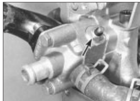
7.12 Temperature sensor (arrowed) - 1.05 and 1.3 litre
