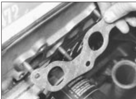
11.19 Fitting a new exhaust manifold gasket
