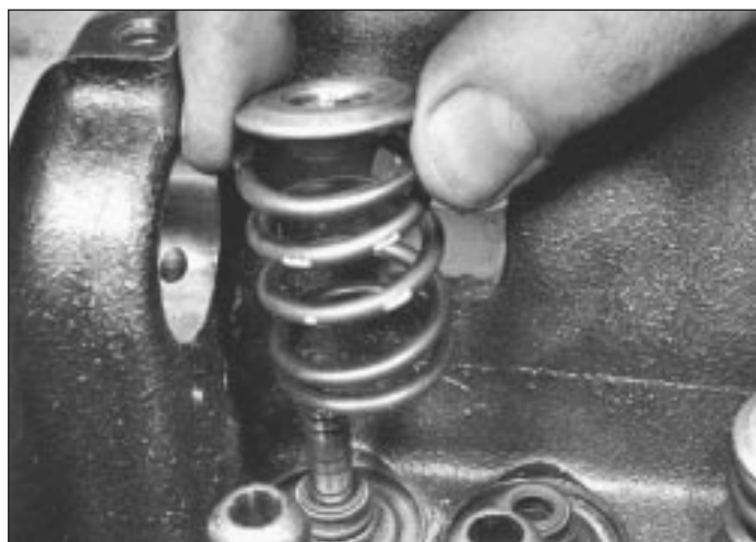
11.2b Removing valve springs and retainers . . .
