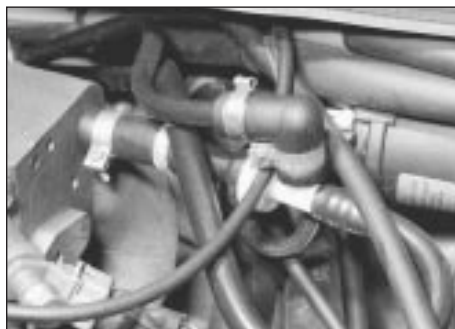
23.5 Vacuum hose-to-cylinder connector
