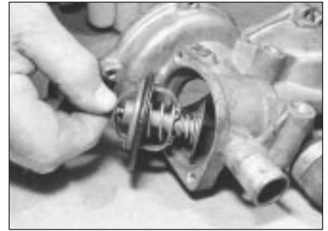
5.11c . . . then extract thermostat and seal
