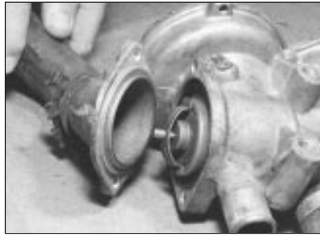
5.11b . . . withdraw thermostat elbow . . .
