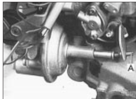
17.39b Fast idle adjustment screw (A)
