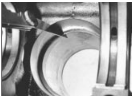
23.6 Checking piston ring gaps
