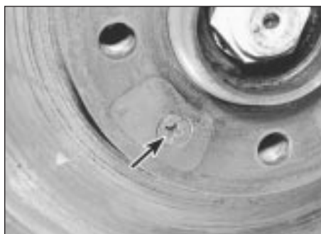
4.5 Front brake disc retaining screw (arrowed)
