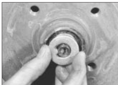
6.5b ... remove the thrustwasher ...
