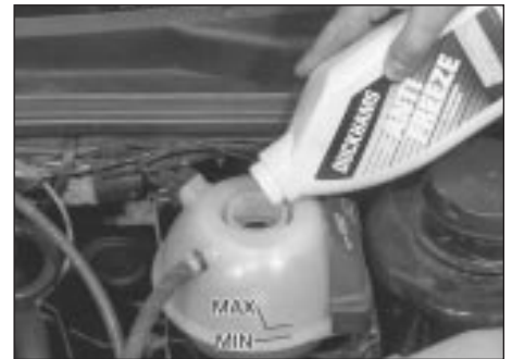
2.13 Topping-up engine coolant
