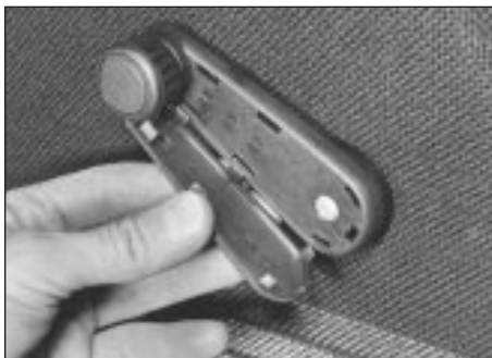
14.4a Remove window regulator handle cover . . .
