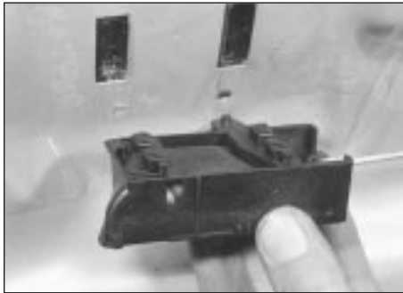
15.3 Removing interior door handle and finger plate
