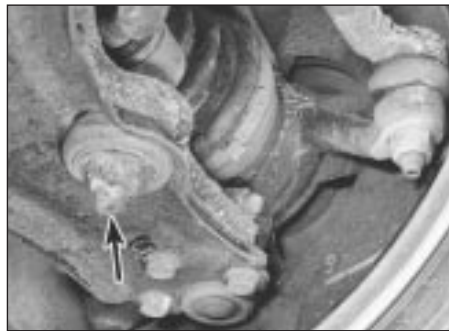
4.2 Anti-roll bar eye bolt nut (arrowed)
