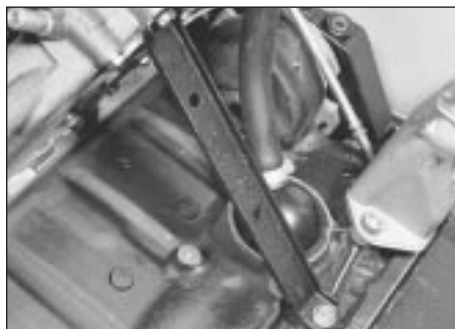
19.5 Inlet manifold support stay - 1.3 litre
