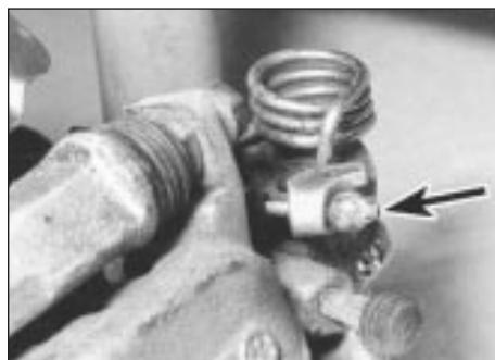
2.15 Release handbrake cable (arrowed) from caliper
