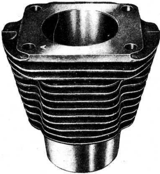
FIG 1:21 Finned cylinder. Letter A stamped on cylinder indicates the class to which cylinder belongs, as referred to its inside diameter
