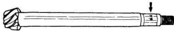
FIG 6:8 Layshaft with final drive pinion. The arrow points to the number (14) for correct mating with ring gear and to the centesimal figure (—10) for accurate mating position of pinion and gear
