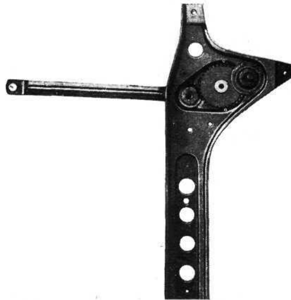
FIG 12:3 Left hand side door window regulator, viewed from car interior
