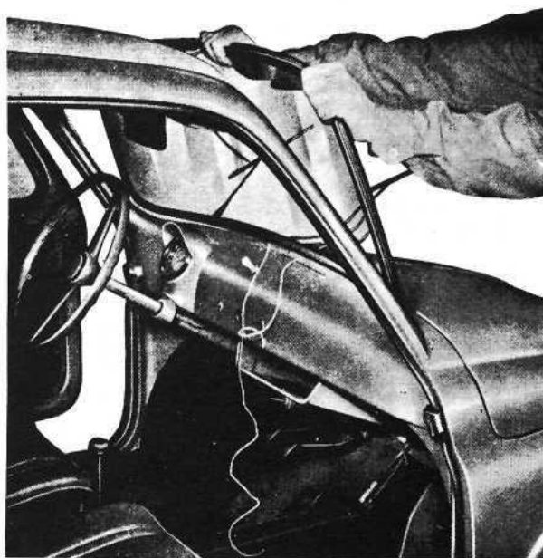
FIG 12:7 Positioning the windshield after tilting wiper blades
